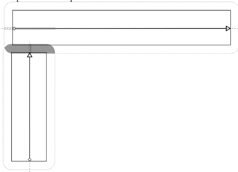
Fig. 2. Graphical depiction of an example wall connectivity intersection operation with two wall “Body” geometries (rectangular); their respective wall “Axis” (a line from square to pointer arrow head); the computed boundary (dotted); boundary intersections (gray); and projections of boundary intersection indicated as narrow rectangle over extended wall “Axis”.
