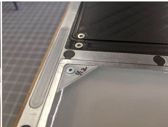
Figure 3.11. Compliant surface test plate corner piece
