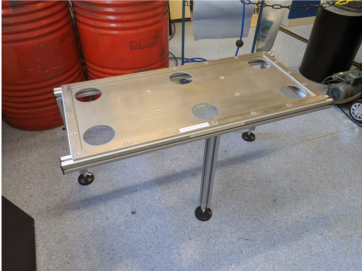
Figure 3.7. The compliant surface mould assembly
