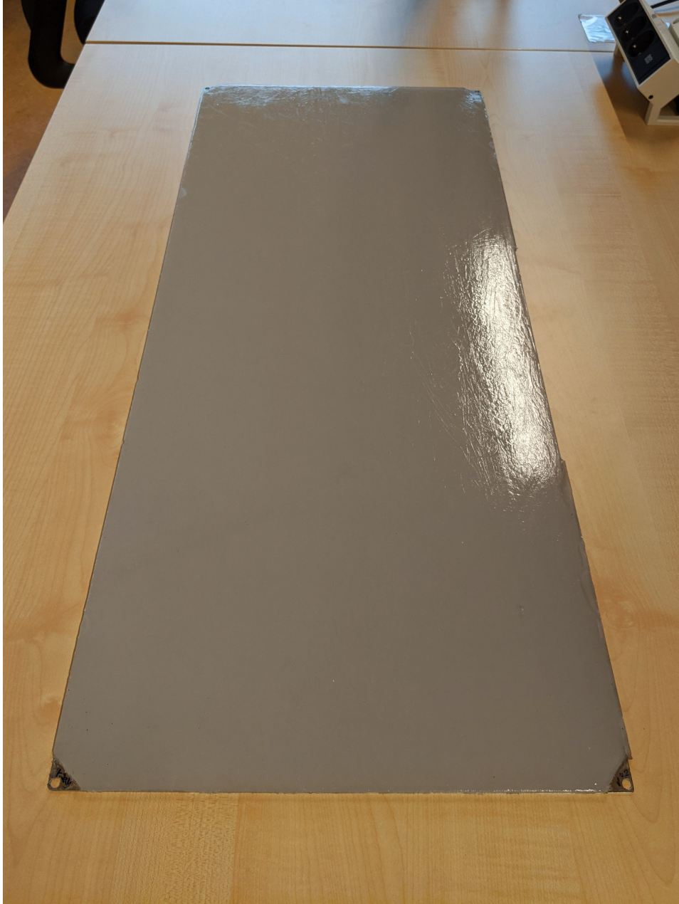
Figure 3.12. A cured compliant surface test plate
