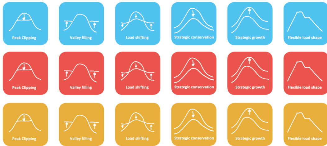
Figure 91: Overview of energy profile effect labels for cooling (blue), heating (red) and supply (yellow)
