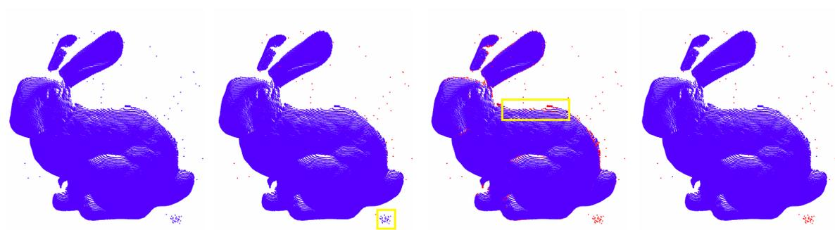
**Figure 3-2:** Comparison between different outlier removal algorithms where red points are labeled as outliers. From left to right: original point cloud, LDOF algorithm where cluster of outliers fails to be detected, NNR algorithm where inliers on manifold border are labeled as outliers, our cluster-adapted algorithm which solves both problems.
