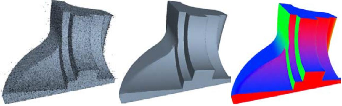
**Figure 2-18:** An example of the MLS fitting method. Left: noisy input cloud. Middle: re-sampling model; Right: middle model colored using normal direction. Figure from Fleishman et al. [30].
