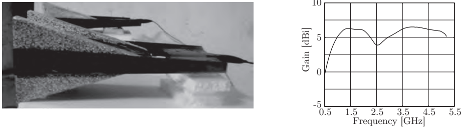
Figure A.6: a) Dielectric wedge antenna; b) Dielectric wedge antenna gain vs. frequency.
