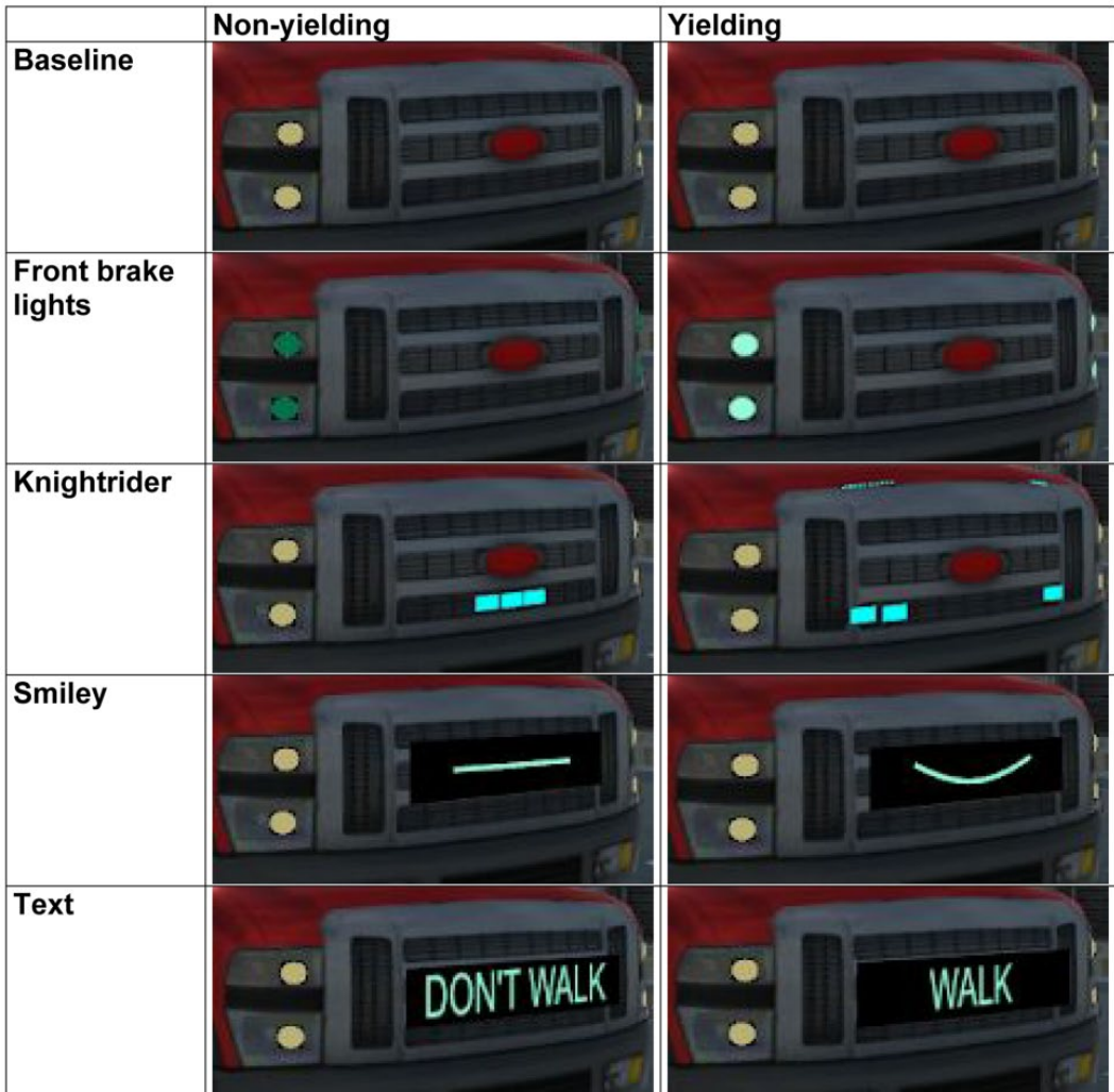
Figure 5. From top to bottom: (1) baseline, (2) front brake lights, (3) Knightrider (in the yielding state, the bar moved from left to right, from the perspective of the participant), (4) smiley, and (5) text.
