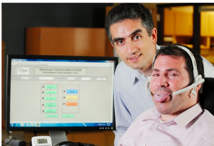
Figure 8 Tongue-movement-based interfaces. The tongue-movement-based interface developed by [76]. This system has two inductive coils mounted at the lateral parts of the mouth and a ferromagnetic material attached at the tip of the tongue. The users generate control commands by moving the tongue to one of the user-defined locations. Tongue movement interfaces take advantage of the fact that highly paralyzed patients generally have tongue control and they can move it very rapidly and accurately within the oral space. Additional file 6 shows a SCI patient performing a driving task with a wheelchair that is controlled with this tongue-movement-based interface. Figure courtesy of Dr. Maysam Ghovanloo.
