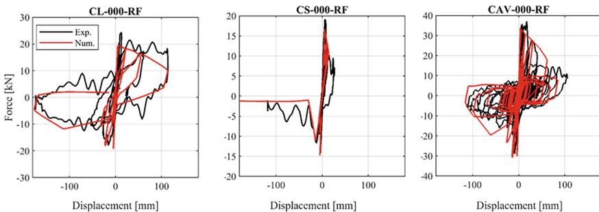
**Fig. 3.** Comparison of numerical and experimental force-displacement hysteresis.
