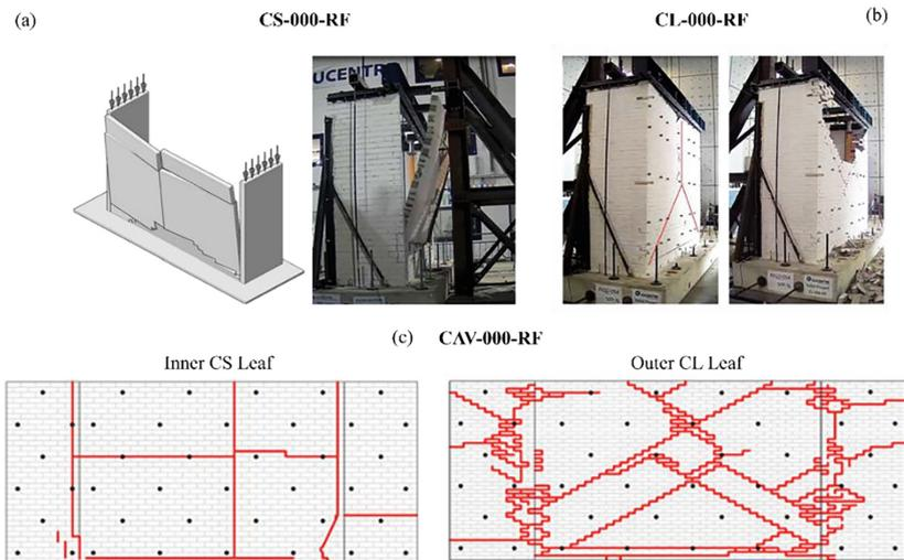
**Fig. 1.** Failure mechanisms of walls (a) CS-000-RF; (b) CL-000-RF and (c) CAV-000-RF observed experimentally.
