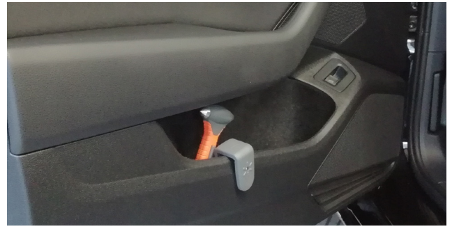
Figure 1.17: Bad placement by Volkswagen mechanic; this hammer could not be removed
