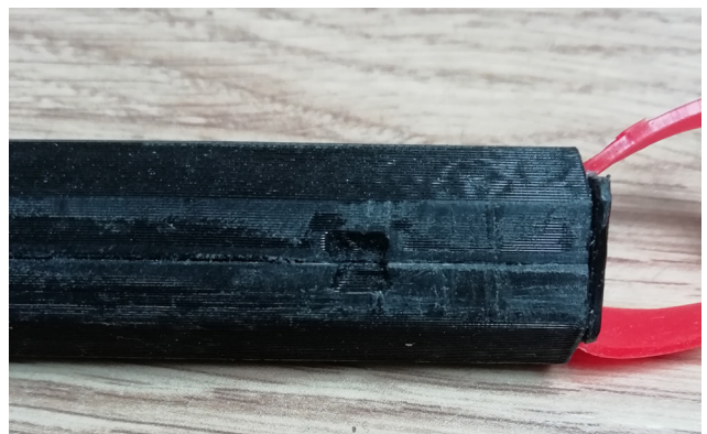
Figure 3.16: Cavity for snap fit
