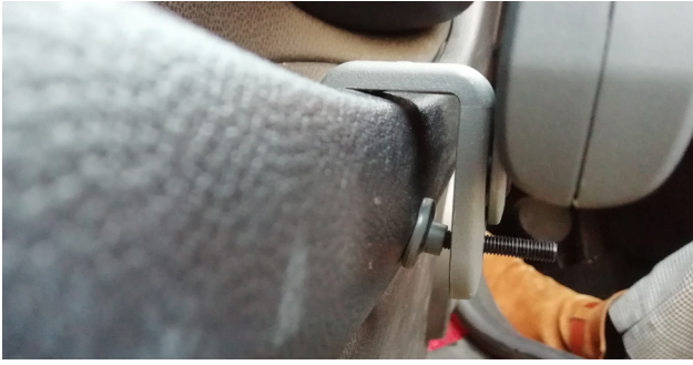
Figure 1.16: Note the stress on the force distributor, as well as the bolt sticking out
