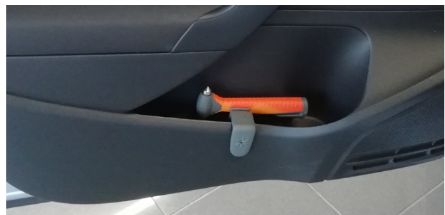
Figure 3.26: UV discolouration on the TPU of a Plus hammer
