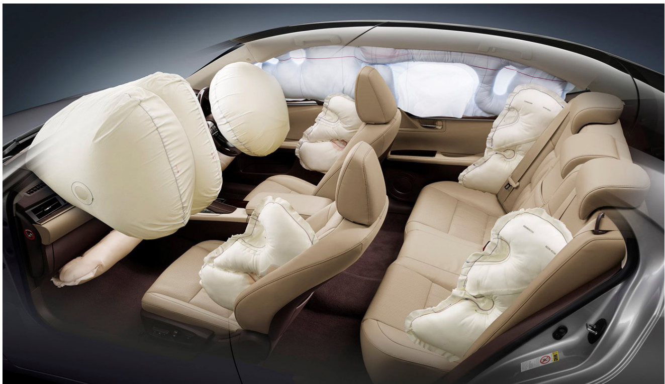
Figure 1.28: Several places where airbags can be found. Source: whichcar.com.au
