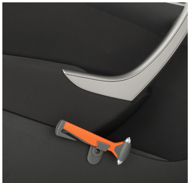
Figure 1.15: The QCS and its location. Note: the bolt is on the interior of the side pocket, which makes it hard to tighten.
