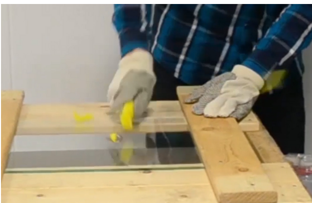
Figure 1.11: Screen shot of a footage of a failing hammer
