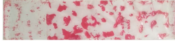
b. Sleeper-ballast contact area with the USPs
