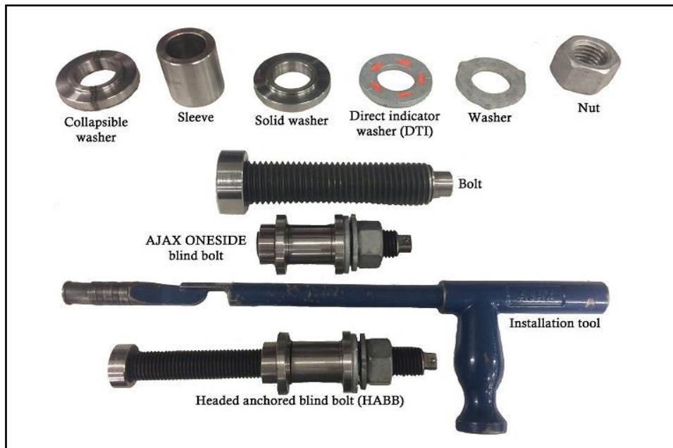
Figure 2-4: Ajax one side bolt
