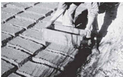
Figure 2.2. Manual production of adobe bricks.
