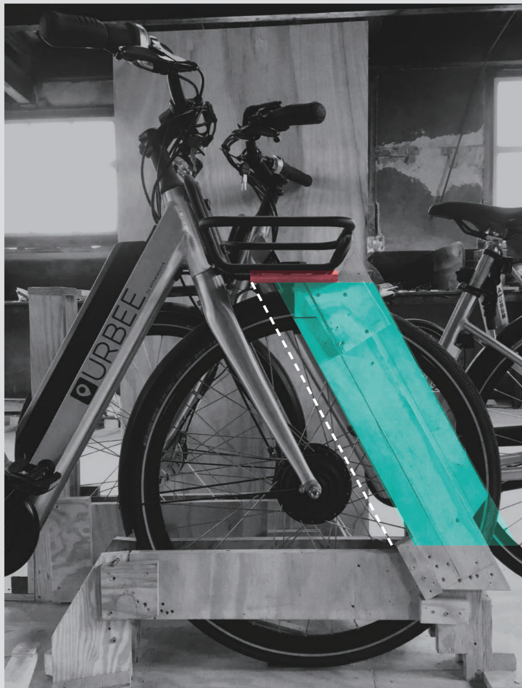
figure 42. prototype to proof the "hanging" concept/ validation the request dimension of charger
