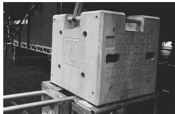
figure 9. concrete anchor with multiple functions (Anchorbloc Ltd, 2017)
