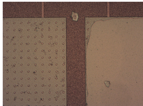
Figure 5-27: Delamination of M2 electrodes after deposition of SiC3 membrane.
