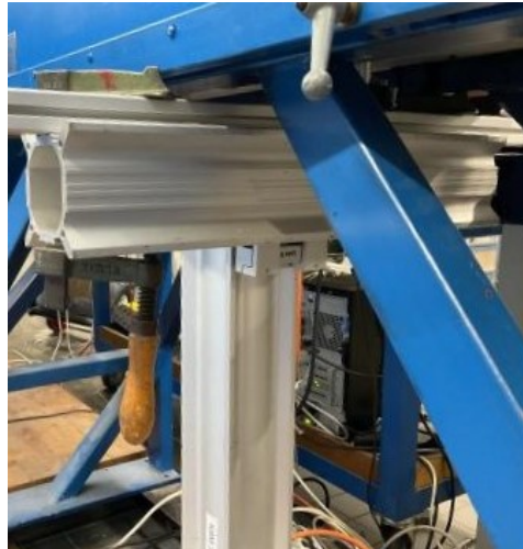
Figure 3.19: Aluminium profile strut clamped on support X beam.
