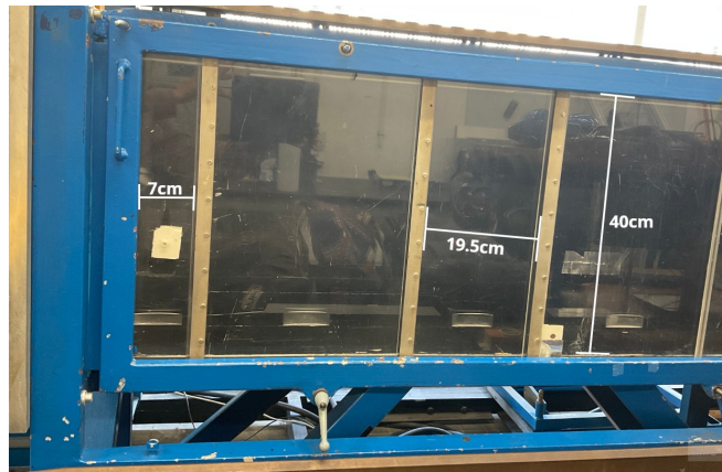
Figure 3.12: Side view and measurements of wind tunnel.
