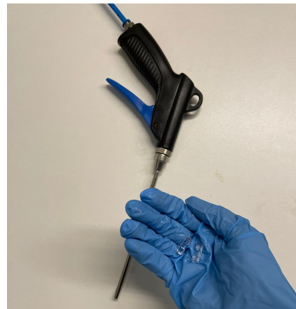
(b) Air-gun for clearing loose openings.
