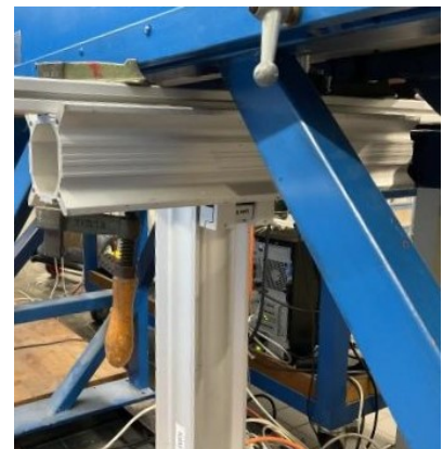
(c) Support rod clamped onto X beam.
