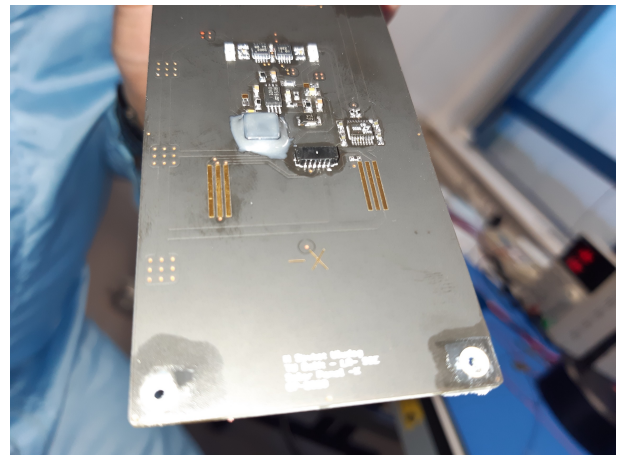
Fig. 27: Spring-loaded contact pads after vibration testing, showing no visible sign of wear.
