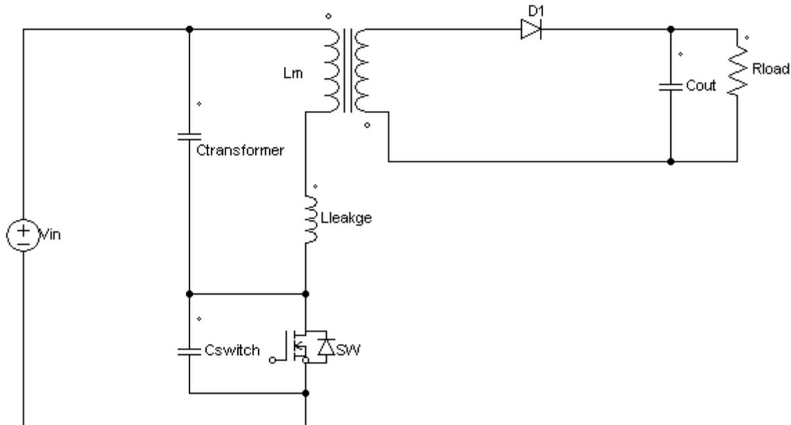
Figure 2 Flyback Model including parasitic elements
