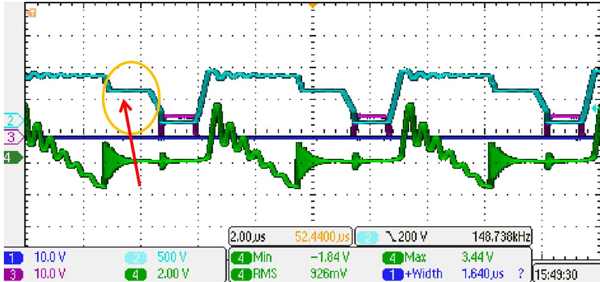
Figure 36 Shows the waveforms of proposed voltage clamping technique under light load condition where the voltage over the switch is shown in blue, the gate voltage of the primary FET is shown in red and the secondary current is shown in green.
