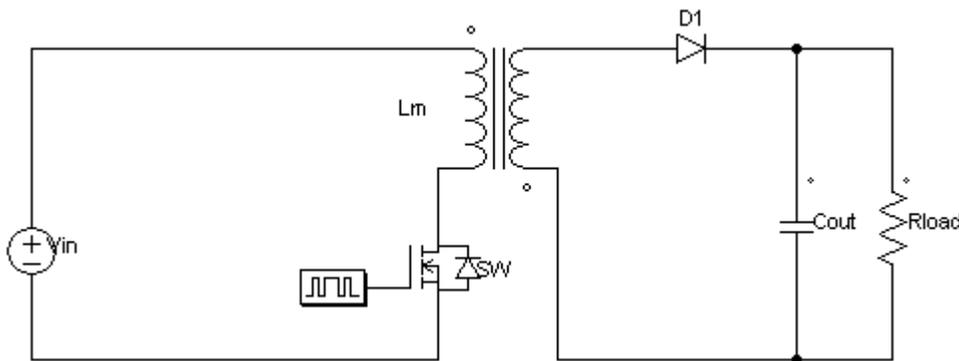
Figure 1 simple schematic of a Flyback converter .
