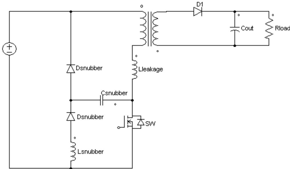
Figure 5 A typical scheme of LC snubber in a Flyback converter
