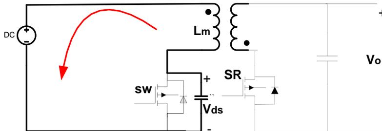
Figure 23 Equivalent circuit during mode 4
