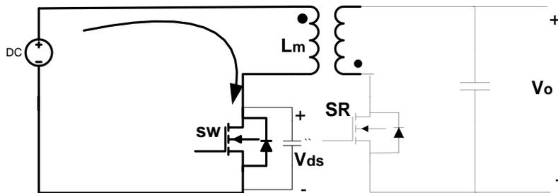
Figure 20 Equivalent circuit during mode 1
