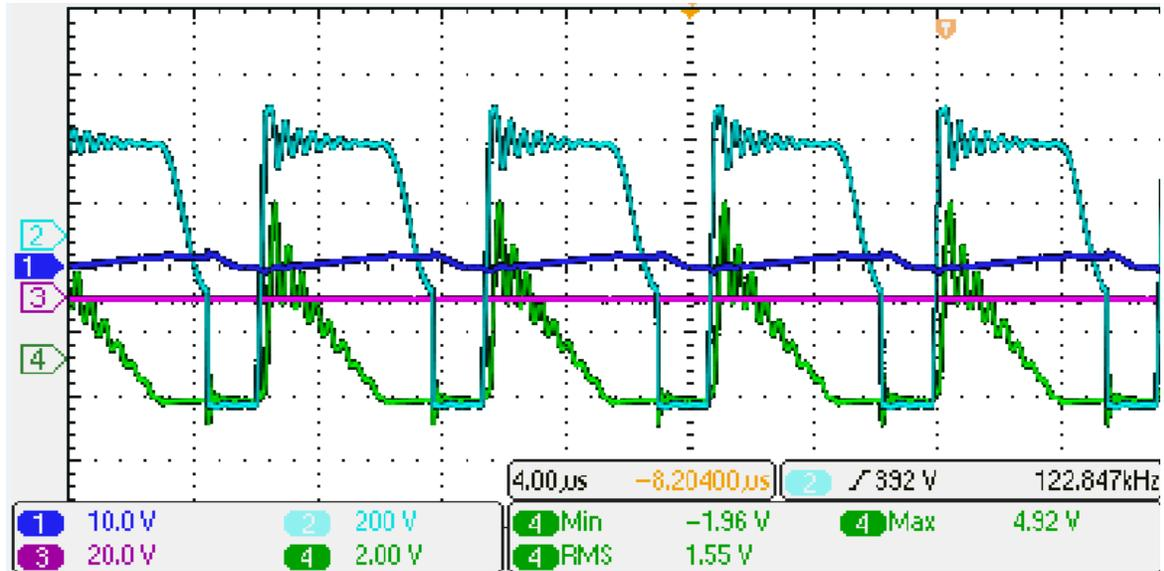
Figure 27 shows the waveforms of “normal” valley switching without reverse current
