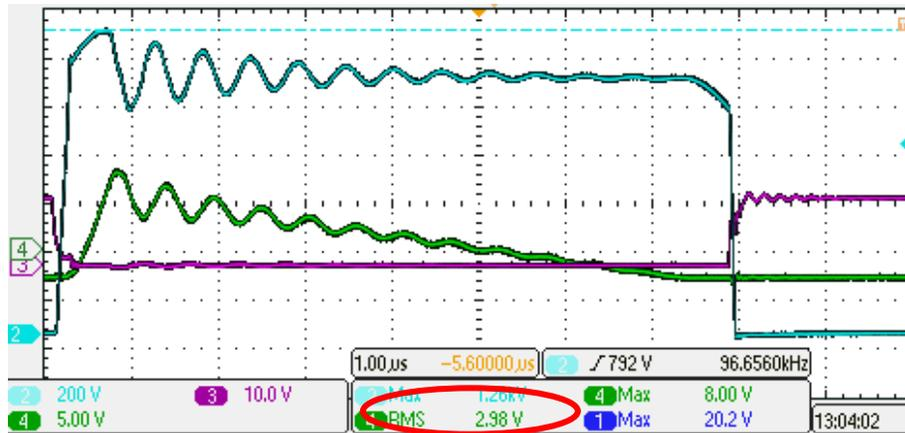
Figure 9 shows the voltage over the switch (blue), the secondary current (green) and the gate voltage winding (purple) with LC snubber
