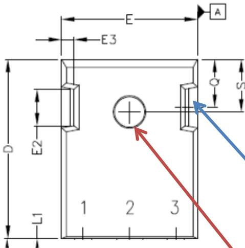
Figure 11 Package dimension of the MOSFET [23]
