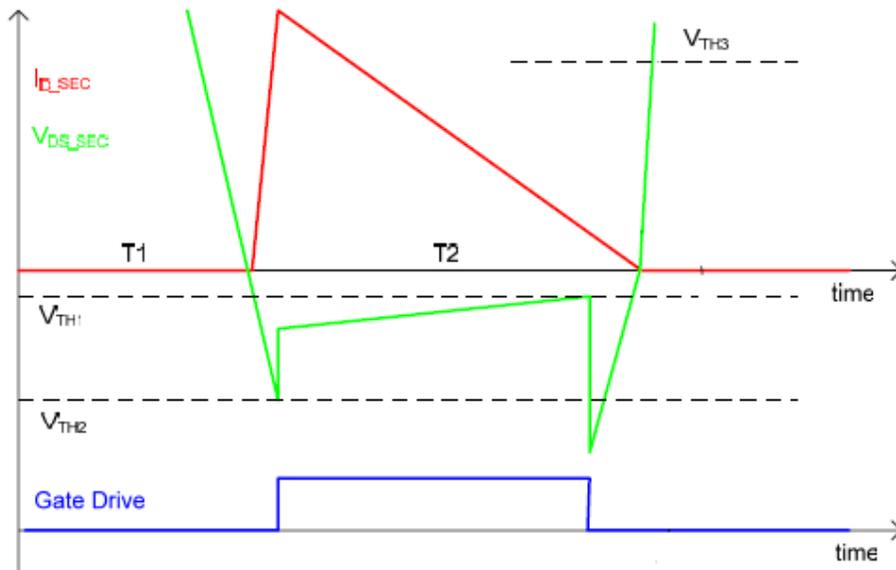
Figure 17 Simplified waveforms of the Flyback converter with SR [22]
