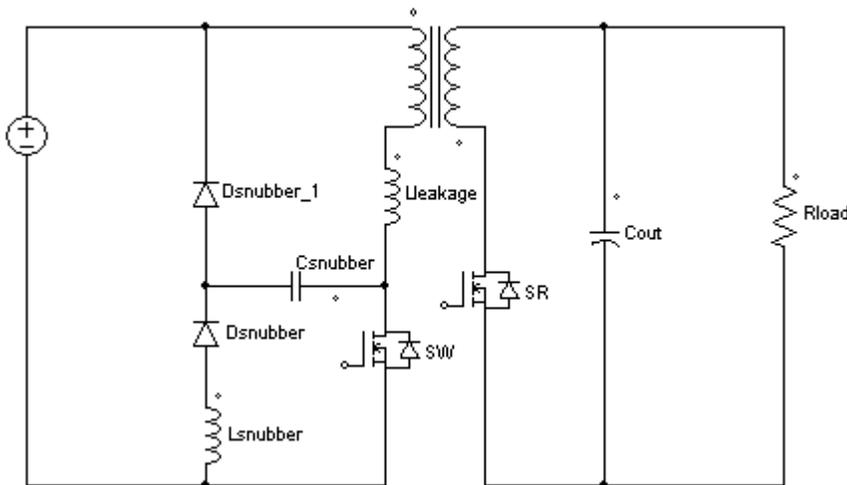
Figure 16 Flyback schematic with LC snubber with SR FET implementation
