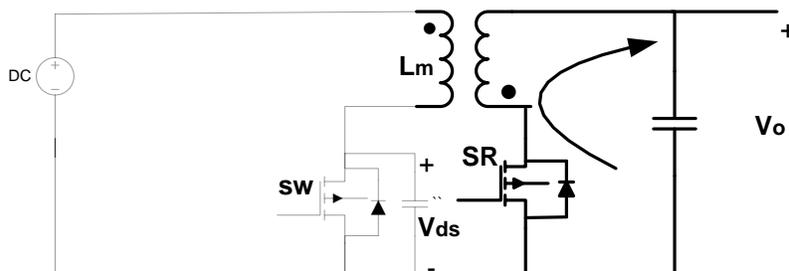
Figure 21 Equivalent circuit during mode 2
