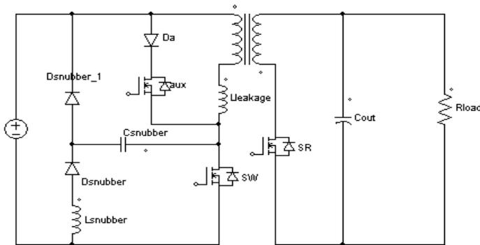
Figure 34 Proposed Flyback circuit with auxiliary circuit based on [25]
