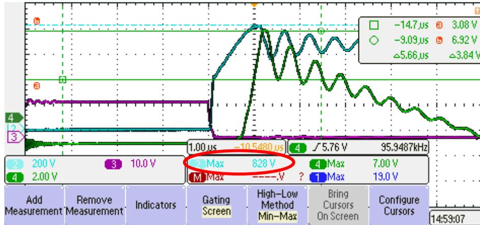
Figure 8 shows the voltage across the primary FET(blue), the secondary current (green) and the gate voltage (purple) with LC snubber implementation
