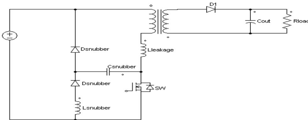
Figure 7 the passive non-dissipative snubber
