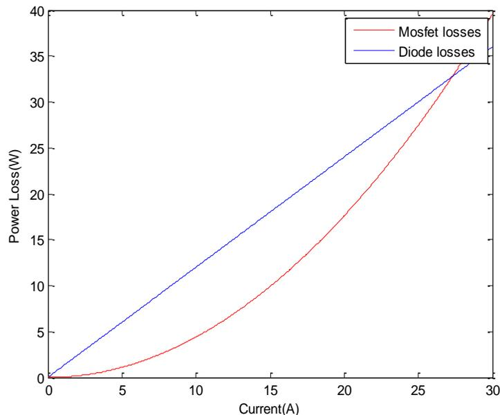
Figure 15 Comparison of the conduction losses in the SR FET and diode as a function of current
