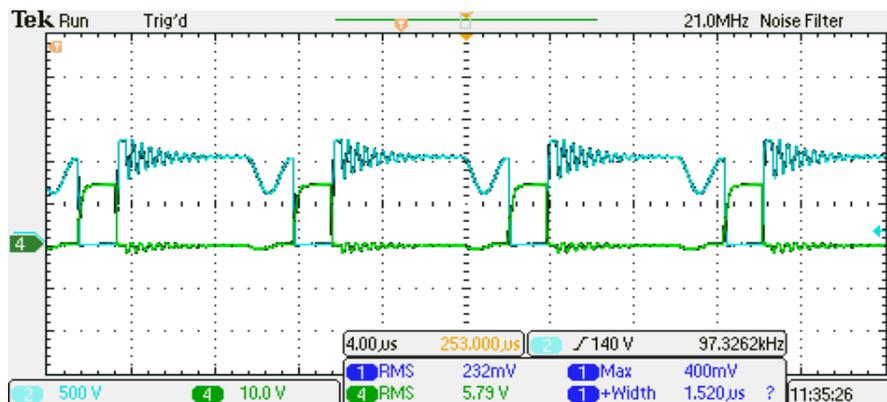
Figure 25 Typical waveforms of valley switching under moderate load condition where the voltage over the switch is shown in blue and the gate voltage of the primary FET is shown in green.
