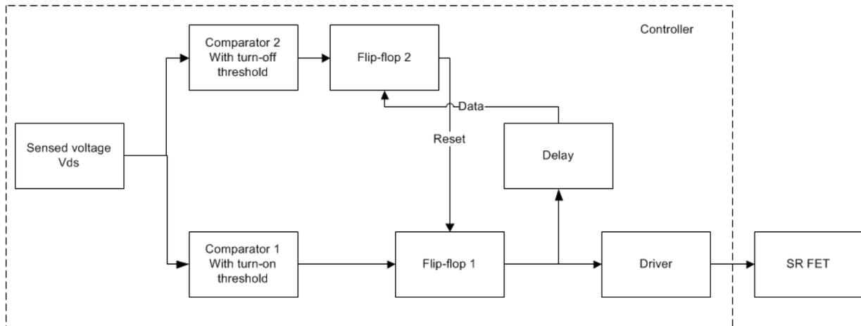
Figure 26 gives an overview of the functional description of the controller
