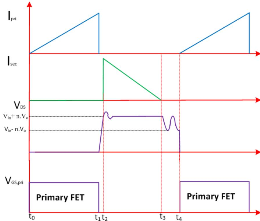
Figure 3 Shows the waveforms during steady state operation of Flyback in DCM
