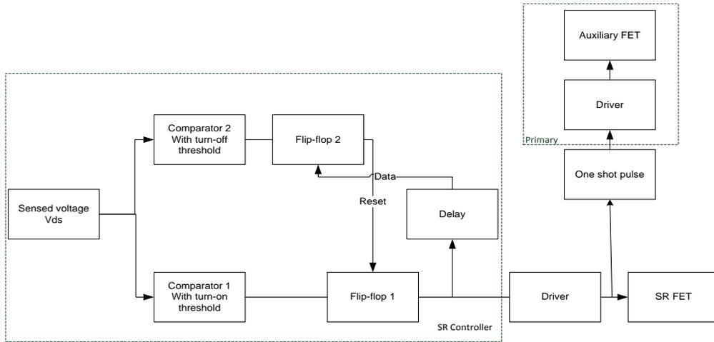
Figure 35 gives an overview of the functional description of the proposed controller with an auxiliary transistor
