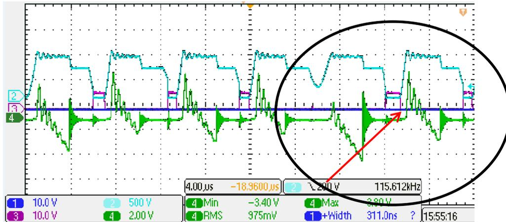
Figure 38 Shows the waveforms of proposed voltage clamping technique with erratic behavior where the voltage over the switch is shown in blue, the gate voltage of the primary FET is shown in red and the secondary current is shown in green.
