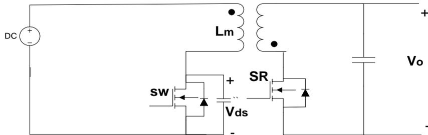
Figure 19 Simplified Flyback circuit with SR
