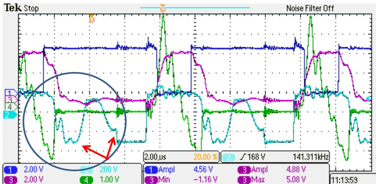
Figure 33 Shows the waveforms at a typical light load condition indicating the effect of the blanking time where the voltage over the switch is shown in blue and the secondary current is shown in green.
