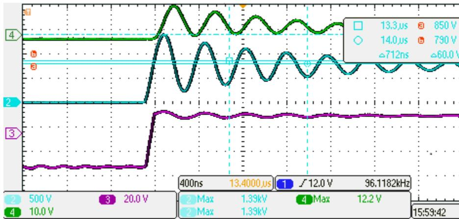
Figure 6 shows the voltage over the switch (blue), the secondary current (green) and voltage over the secondary winding (purple) without interleaving. Note how the peak voltage is almost 1400V with minimum input voltage
