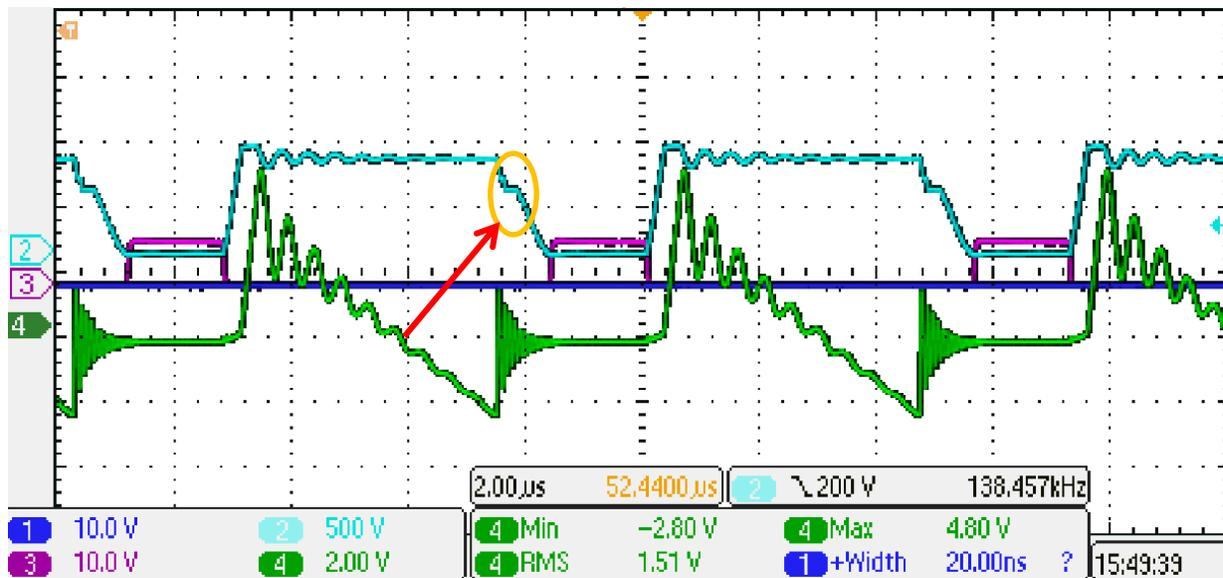
Figure 37 Shows the waveforms of proposed voltage clamping technique under moderate load condition where the voltage over the switch is shown in blue, the gate voltage of the primary FET is shown in red and the secondary current is shown in green.
