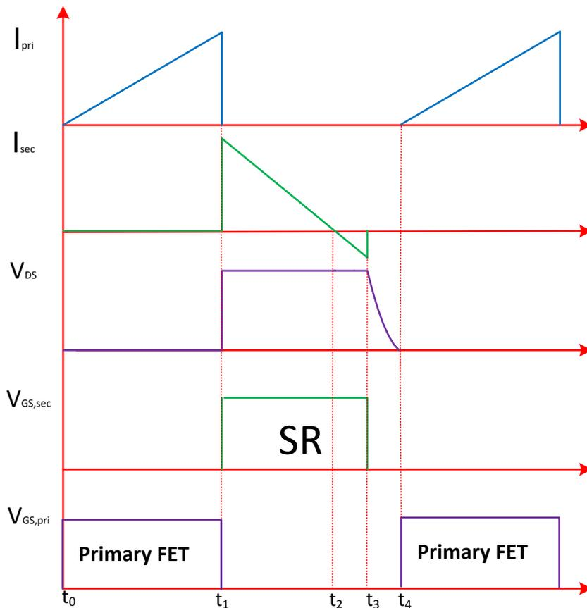
Figure 18 Shows the waveform during steady state operation of the Flyback with SRMT
