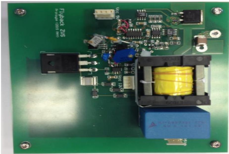
Figure 29 Shows the Flyback converter with the proposed controller implemented on PCB
