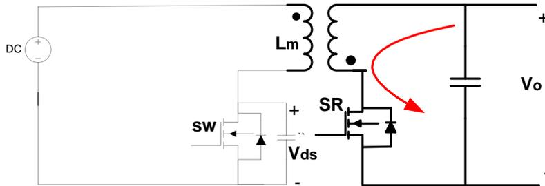
Figure 22 Equivalent circuit during mode 3
