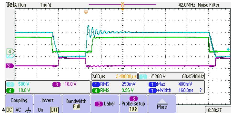
Figure 32 Shows the results of the proposed ZVS scheme at full load and 800V input voltage implemented on the PCB where the voltage over the switch is shown in blue, the gate voltage of the primary FET is shown in red and the gate voltage of the SR FET is shown in green.
