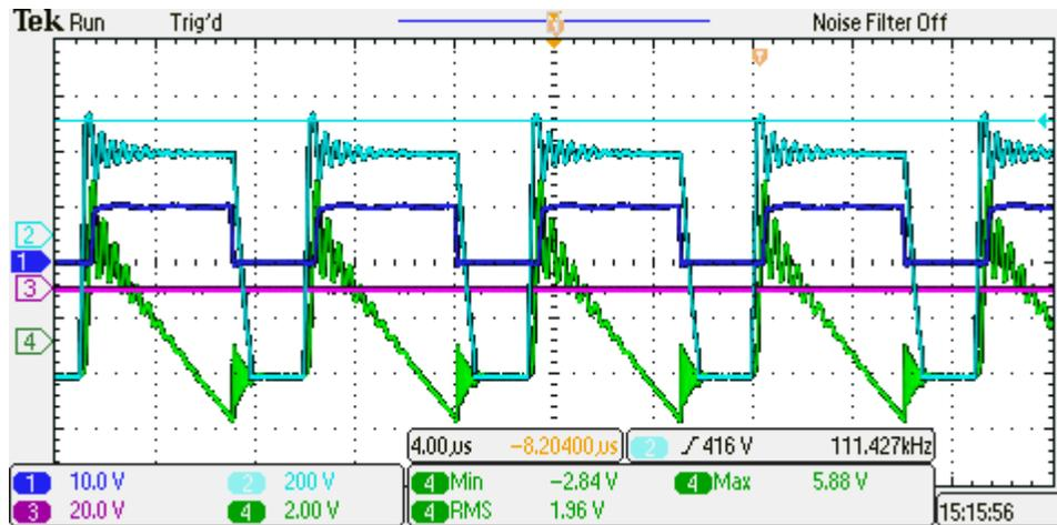
Figure 30 Shows the experimental results of the proposed ZVS scheme implemented on the protoboard where the voltage over the switch is shown in blue , the gate voltage of the SR FET is shown in blue and the current is shown in green
