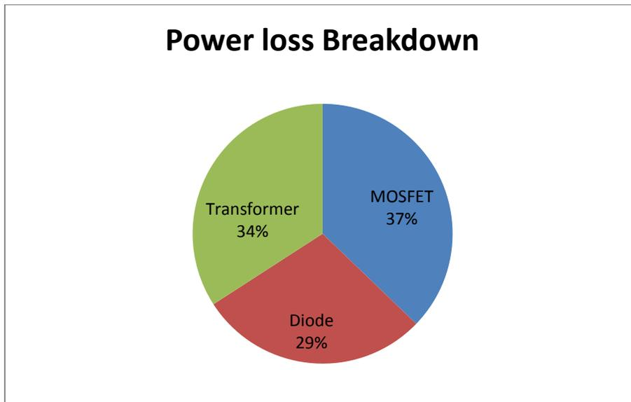
Figure 14 Power loss breakdown of the different components
