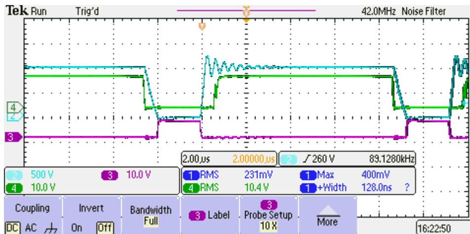
Figure 31 Shows the results of the proposed ZVS scheme at full load and 400 input voltage implemented on the PCB where the voltage over the switch is shown in blue, the gate voltage of the primary FET is shown in red and the gate voltage of the SR FET is shown in green.
