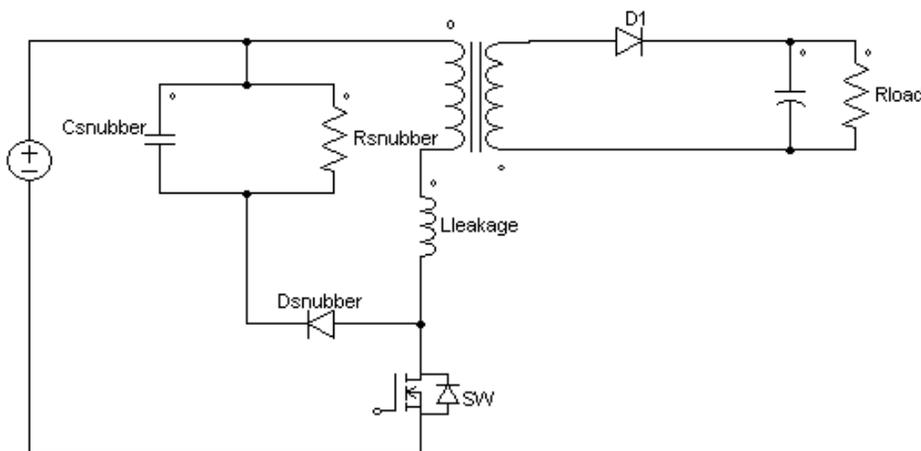
Figure 4 A typical scheme of a RCD Snubber in a Flyback converter
