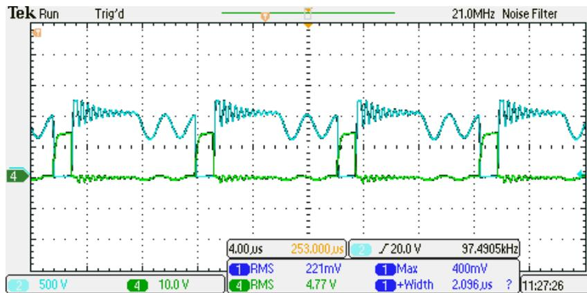
Figure 24 Typical waveforms of valley switching under light load condition where the voltage over the switch is shown in blue and the gate voltage of the primary FET is shown in green.
