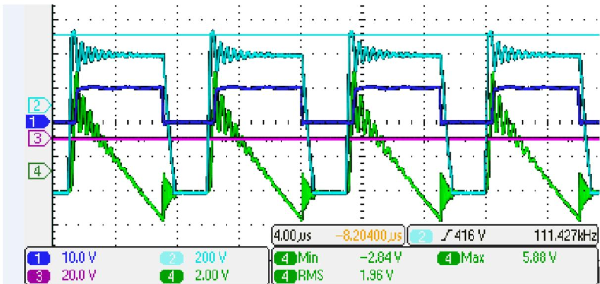
Figure 28 Shows the waveforms of ZVS by allowing the current to go negative
