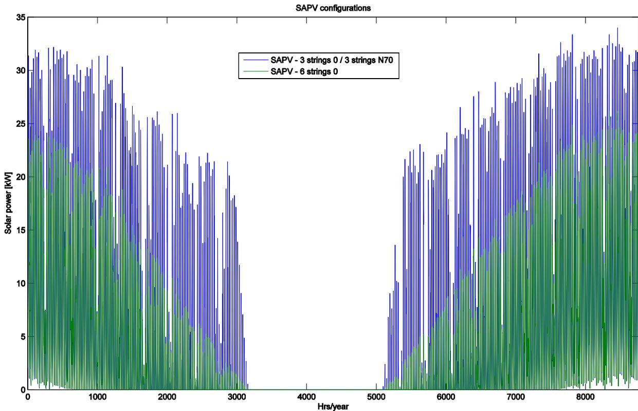
Figure 17: Yields original versus reoriented SAPV
