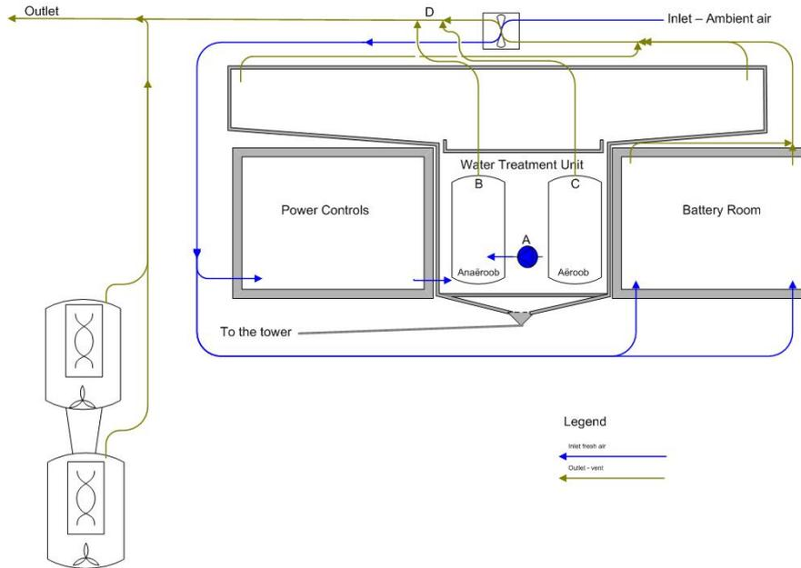
Figure 69: Layout ventilation – technical core
