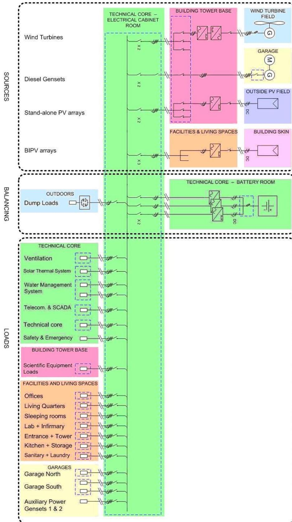
Figure 20: Principle schematic electrical systems [14]
