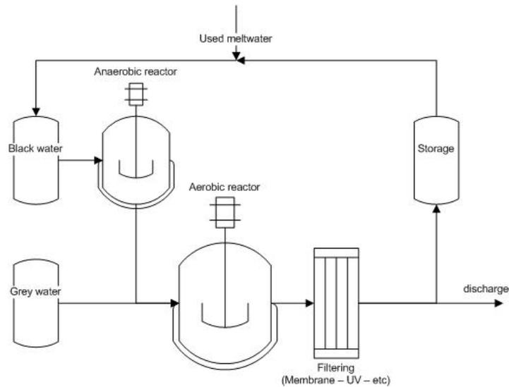
Figure 12: Schematic overview water treatment unit (WTU)
