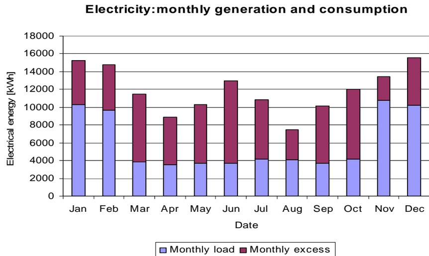
Figure 23: Summer station - electricity: monthly load and excess
