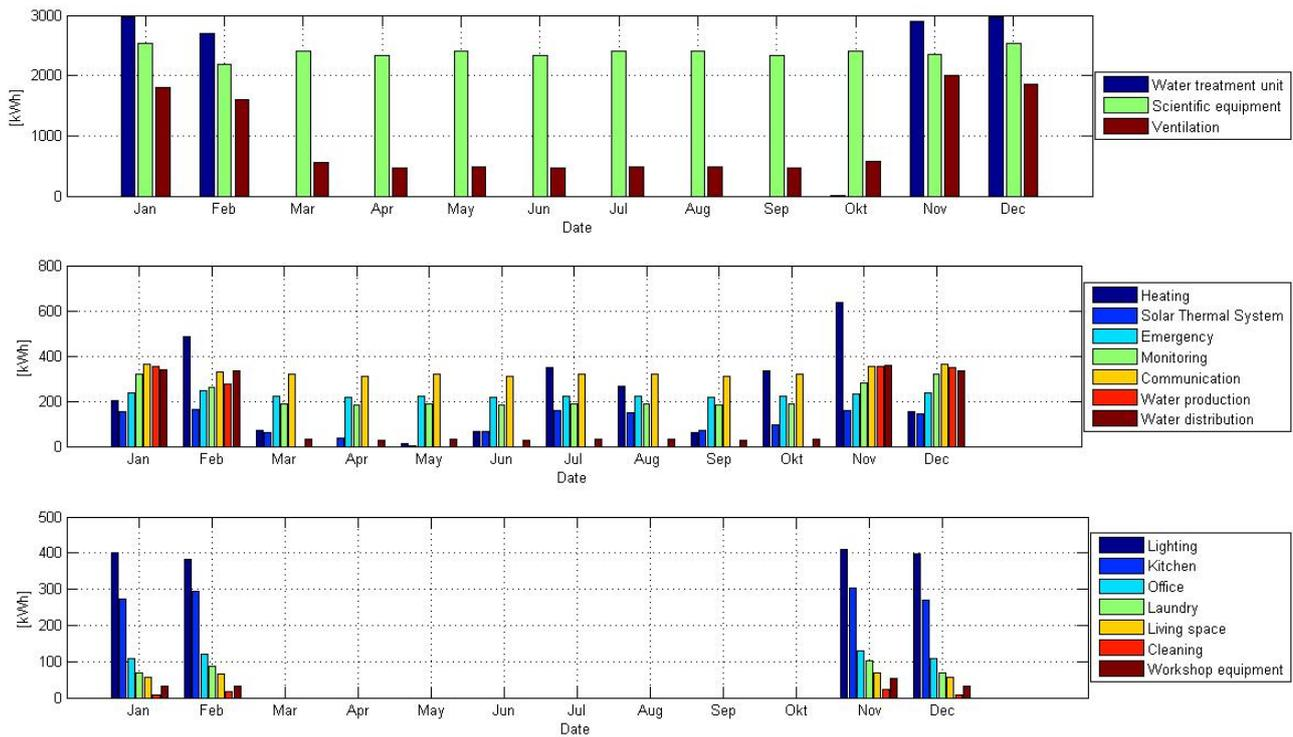
Figure 13: Monthly electrical energy consumption
