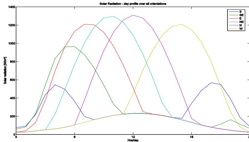
Figure 78: Radiation day profile BIPV (21 November)
