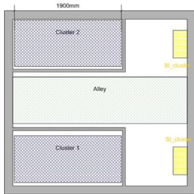
Figure 86: Battery trade-off 1: AGM - layout battery room
