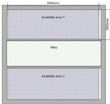
Figure 87: Battery trade-off 2 – final layout battery room
