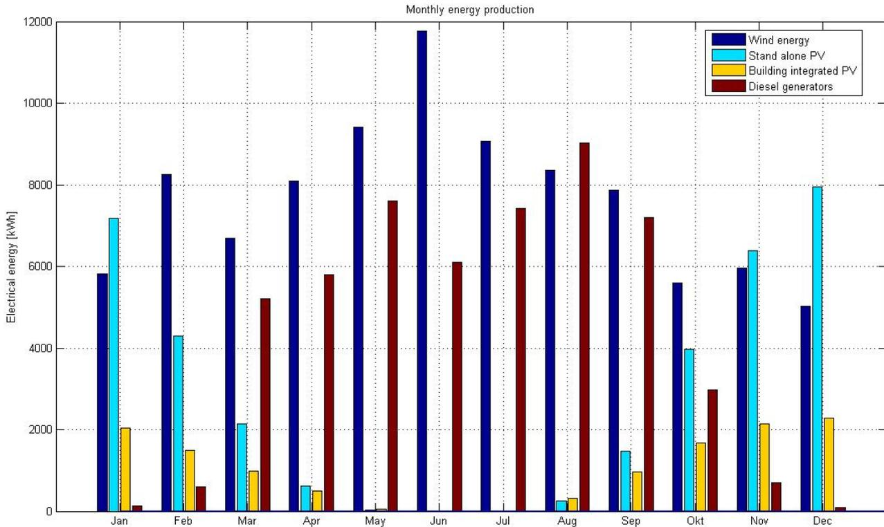
Figure 39: Permanent station - sources - monthly production (potential)
