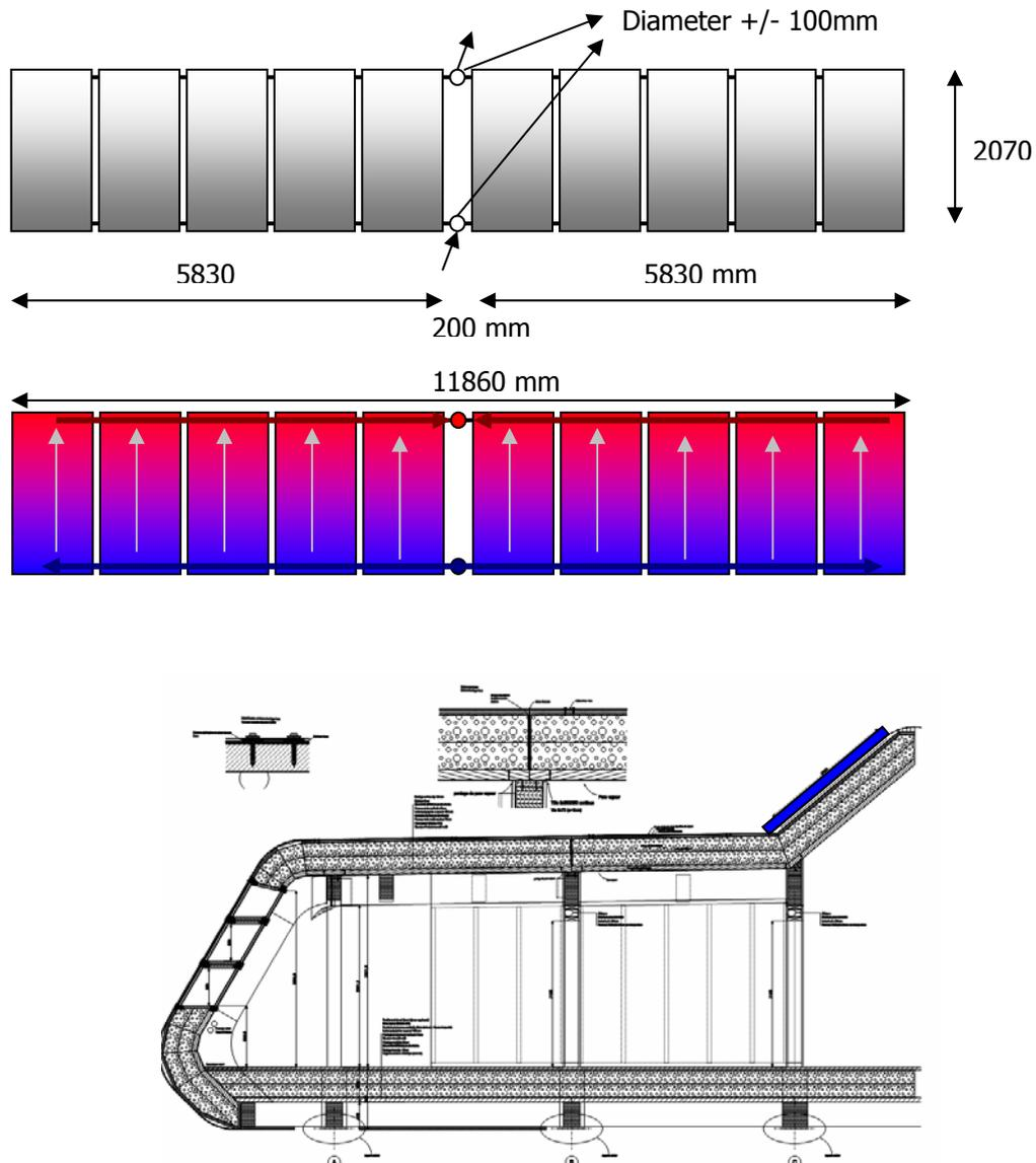
Figure 83: Integration of solar collector on the building skin
