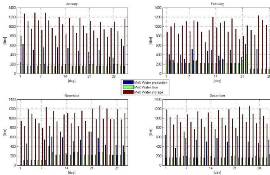
Figure 66: Meltwater production, storage & use
