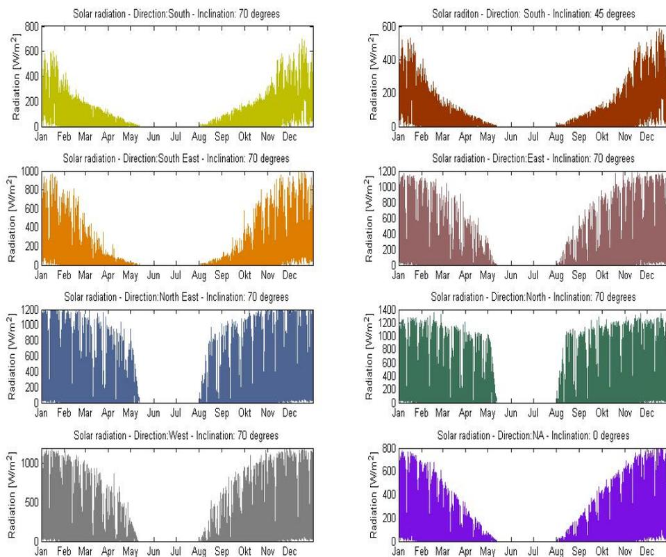
Figure 77: Solar radiation on building (TRNSYS)
