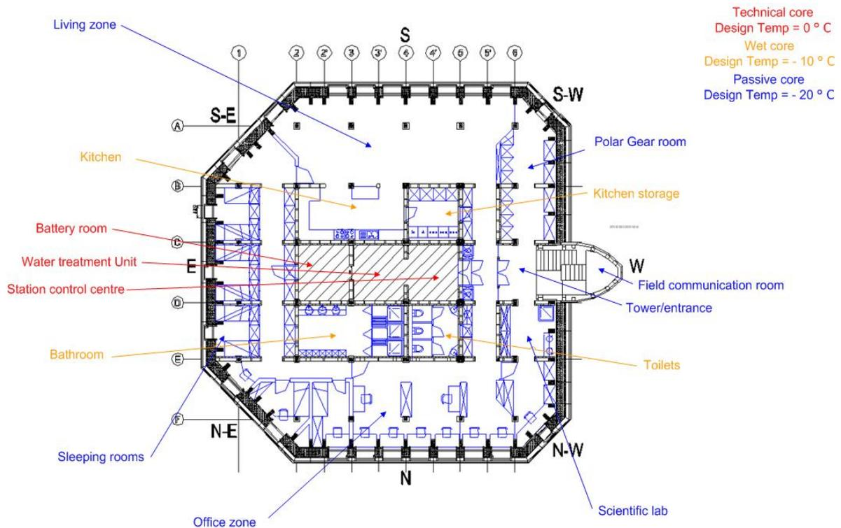
Figure 6: Building layout (dimension: 22 x 22 m) [1]
