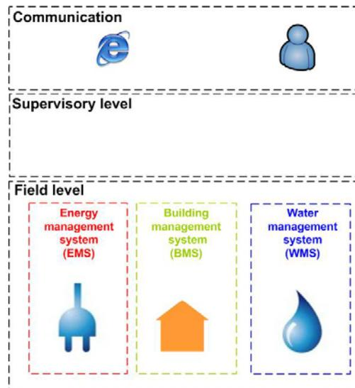
Figure 21: SCADA structure
