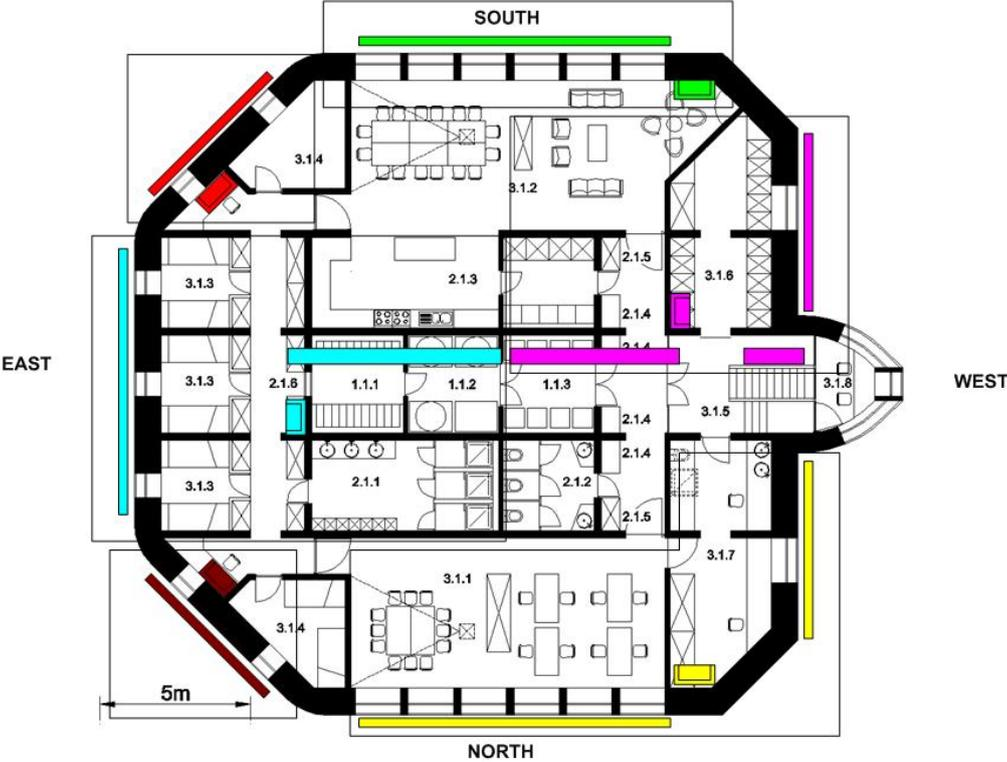
Figure 82: Array configuration BIPV
