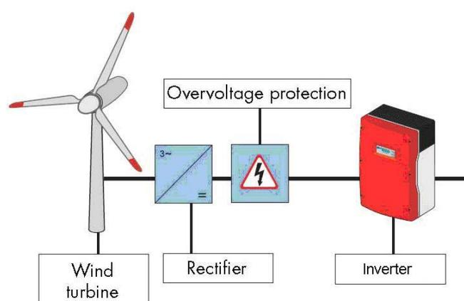
**Figure 14: Rectifier and inverter for wind turbines [51]**
