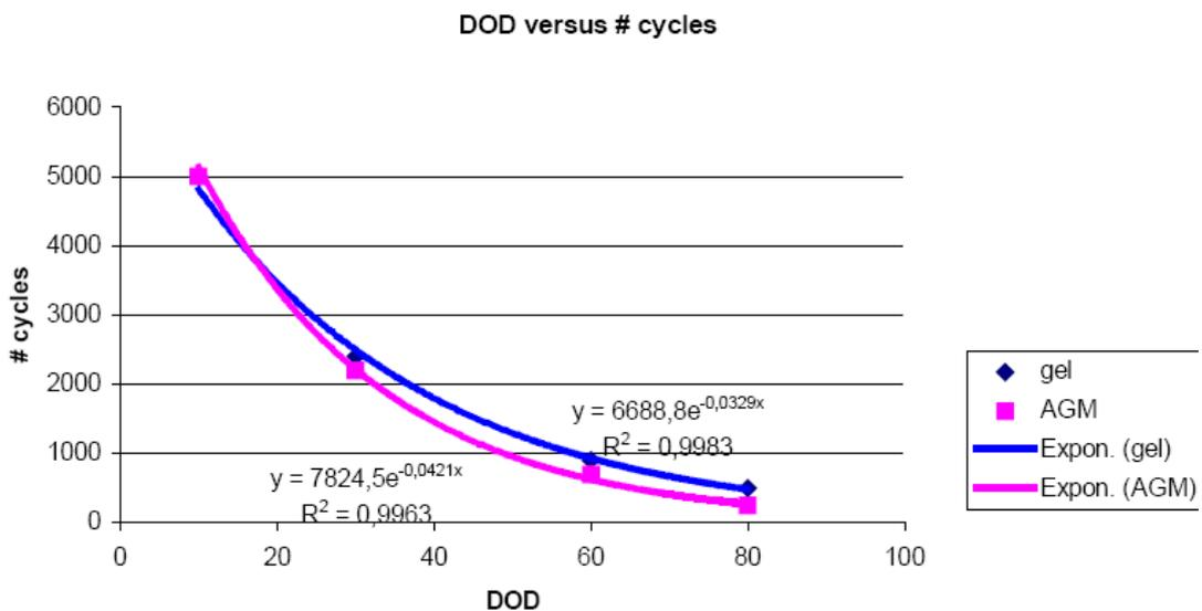
Figure 88: Lifetime estimation curve AGM / Gel
