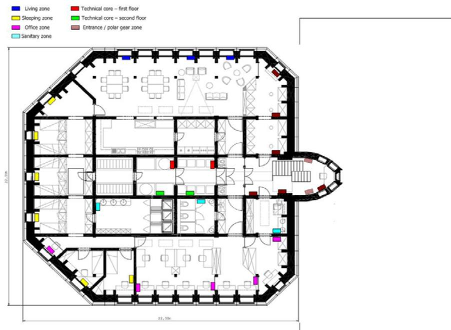
Figure 67: Layout of decentralised heating elements
