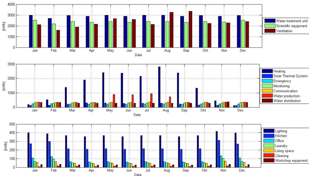
Figure 38: Permanent station - sources - monthly production (potential)
