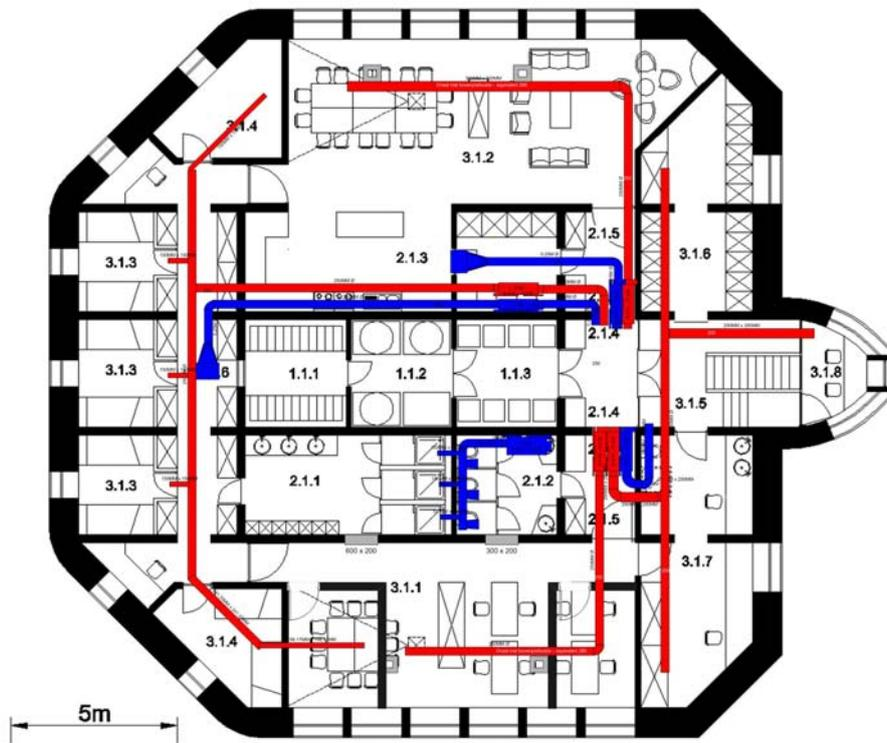
Figure 70: Layout ventilation – wet core and passive zone
