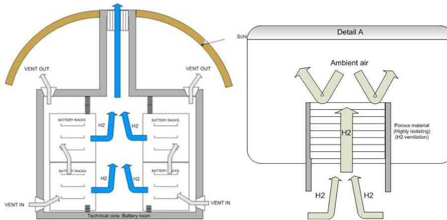
Figure 84: Cross section of ventilation - technical core
