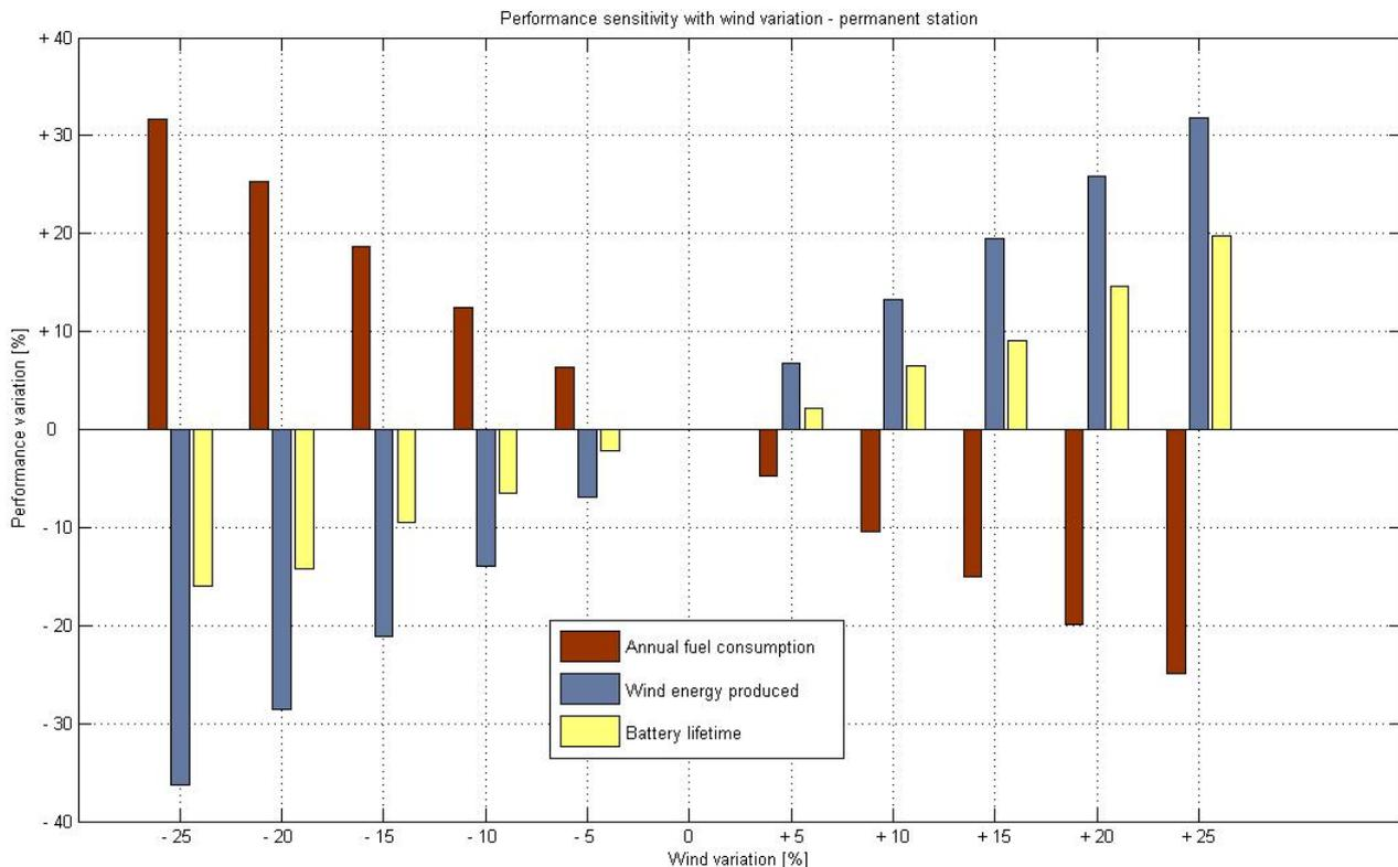
Figure 43: Permanent station - performance sensitivity for wind variation
