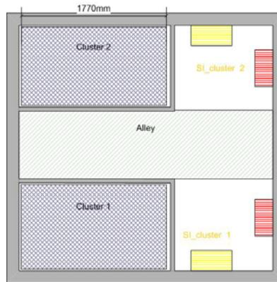
Figure 85: Battery trade-off 1: Gel - layout battery room
