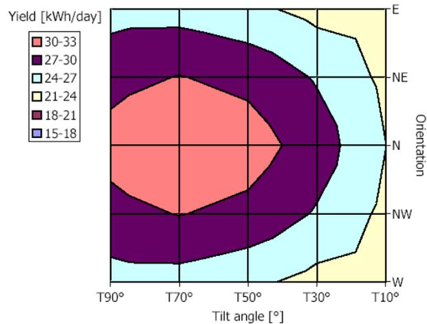
Figure 76: Influence of orientation and tilt angle for a 10 kWp PV system [Source: 3E]
