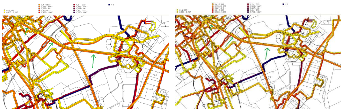
Figure 4.11: I/C ratio during evening peak in case of major discrete event on link segment Laan van NOI - Forepark when no measures are taken (left) and when extra IC stops are temporarily added (right)
