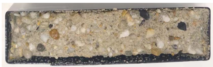
Figure 6.3.3 An AASM with an extreme extent of scaling of around 13 \text{ kg/m}^2 at the end of the CDF test due to the exposure to 55% RH ambient air after demolding. Adapted from [66].
