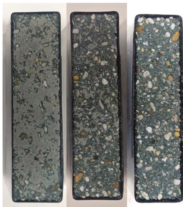
Figure 6.3.2 Surface condition of an AASM during the CDF test, from left to right: 4 cycles, 14 cycles, 28 cycles. Adapted from [66].
