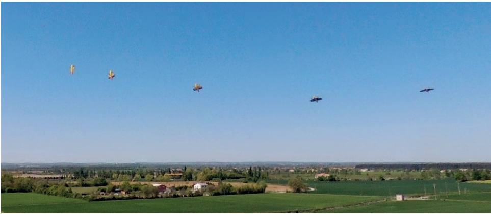
Figure 5.16: Composite image of a transition to hover flight, with 1 s image intervals. Footage was taken with a hovering Bebop.
