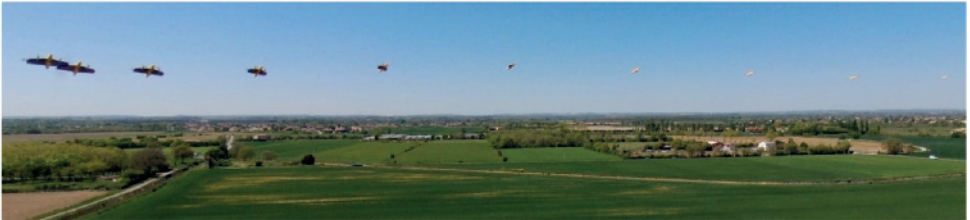
Figure 5.15: Composite image of a transition to forward flight with a constant acceleration of 1 \text{ m/s}^2 , with 1 s image intervals. Footage was taken with a Bebop, which was hovering in place and rotating to keep the drone in the frame.
