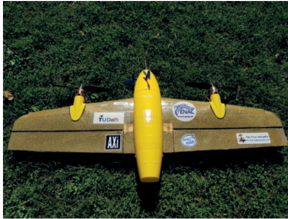
Figure 5.7: The Cyclone with angle of attack and sideslip vanes mounted. The vanes are only used for validation and not for control.
