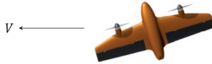
Figure 5.4: Knife-edge flight: hovering with a roll angle to attain a sideways velocity.
