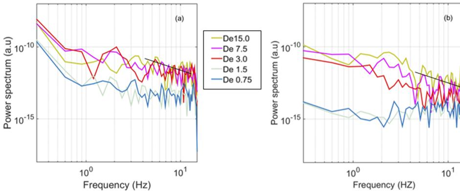
FIG. 5. (a) Power spectrum of stream-wise velocity fluctuations. (b) Power spectrum of lateral velocity fluctuations.
