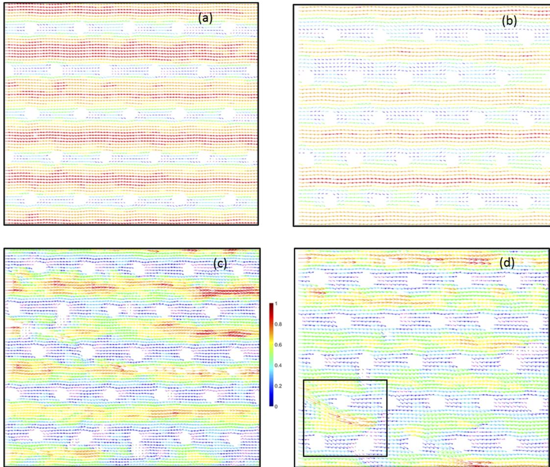
FIG. 7. Time averaged velocity profiles (normalized) at (a)  $De_L$  0.5, (b)  $De_L$  2.0, (c)  $De_L$  3.0, and (d)  $De_L$  10.0 (arrows show the flow direction in the domain, blue to red code shows the lowest to highest normalized velocity magnitude). Average is over 100 successive images.
