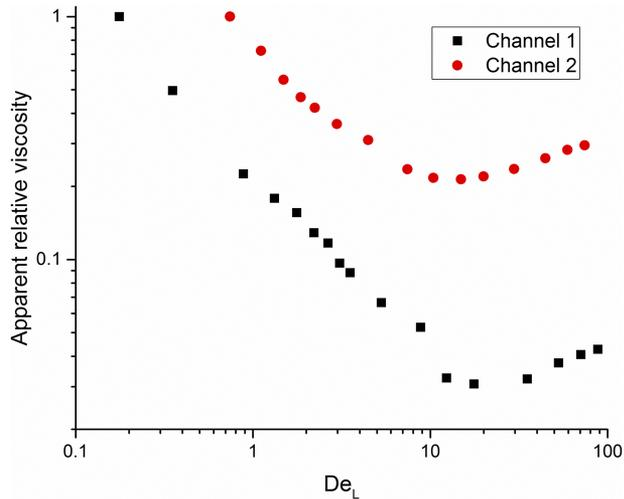
FIG. 8. Plot of normalized pressure drop across the pillared channel as a function of a  $De_L$  number for  $34\ \mu\text{m}$  and  $68\ \mu\text{m}$  channel.
