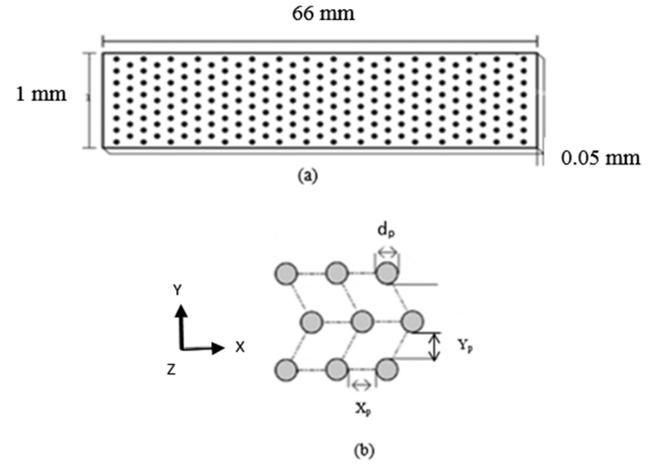
FIG. 1. Schematic drawing of the pillared microchannel. Flow is from left to right ( $x$ -direction). Planar walls are present at both sides in the width ( $y$ ) and height ( $z$ ) directions.
