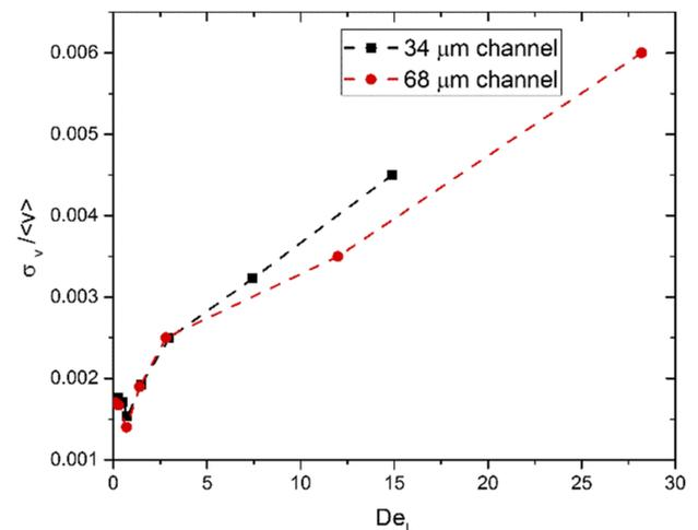
FIG. 6. Time averaged velocity fluctuations vs. Deborah number  $De_L$  total fluctuating magnitude normalized by the average flow velocity for 34 and 68  $\mu\text{m}$  channel.
