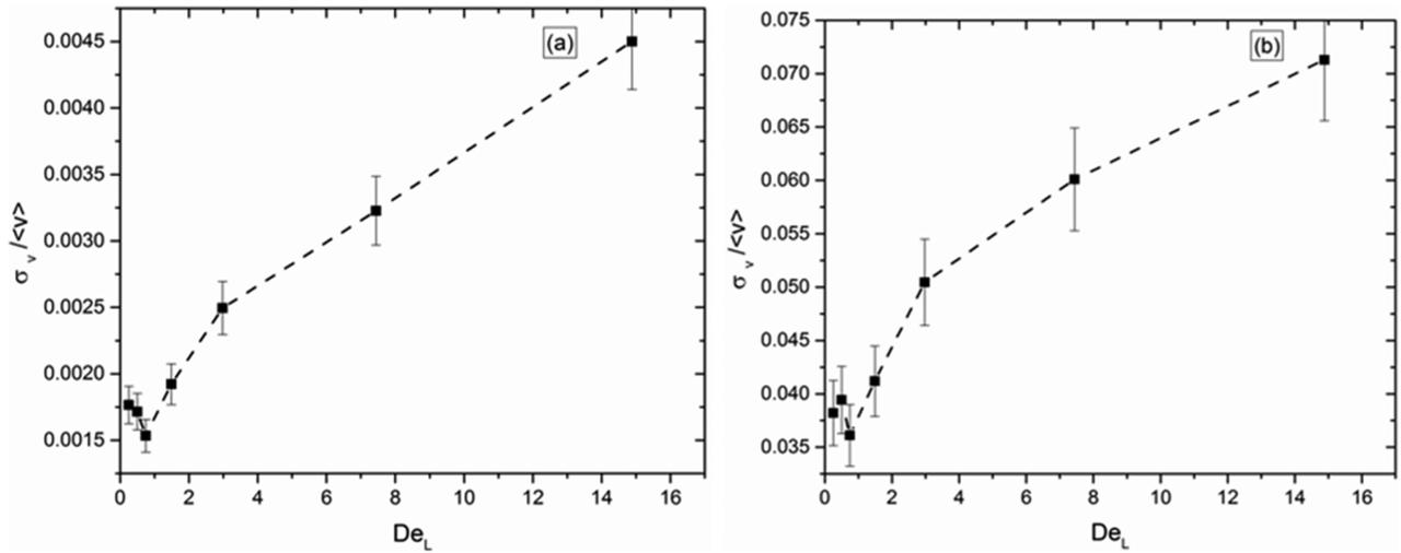
FIG. 3. (a) Time-averaged spatial standard deviation of the velocity normalized by the average flow velocity vs. Deborah number  $De_L$ ; (b) spatially averaged temporal standard deviation of the velocity normalized by the average flow velocity vs. Deborah number  $De_L$ .
