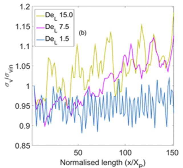
FIG. 4. Streamwise standard deviation of the velocity, normalized by standard deviation at the entrance of the observation region ( $x = 0$ ) as a function of position (normalized by the  $x$ -pitch) along the channel length. Different colors correspond to different Deborah numbers ( $De_L$ ).
