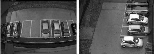
Fig. 3. Parking places (light polygons) selected in video frames from two cameras with different viewing angles
