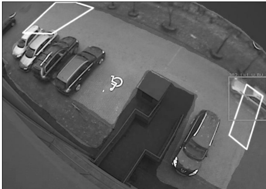
Fig. 1. An example of hot areas placement (white polygons) and a moving vehicle entering the frame in the right hot area (gray rectangle).
