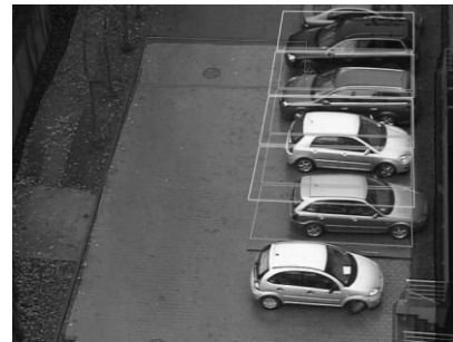
Fig. 4. Lower (gray) and upper (white) bases of 3D right prisms that are used to model four parking place seen in a video frame.
