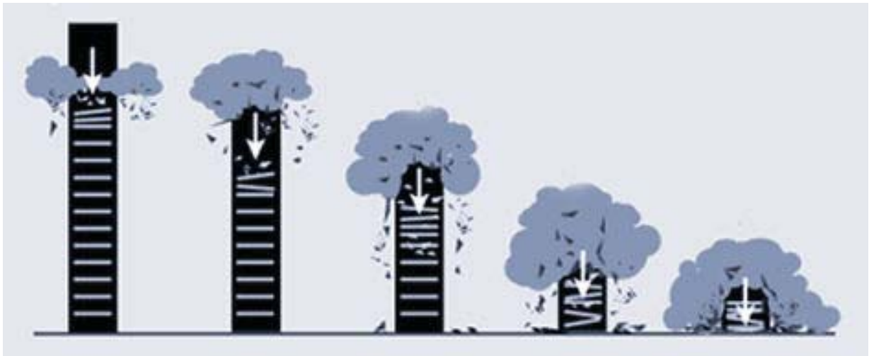
Figure.3.1 Pancake type collapse [Source: http://www.911review.com ]
