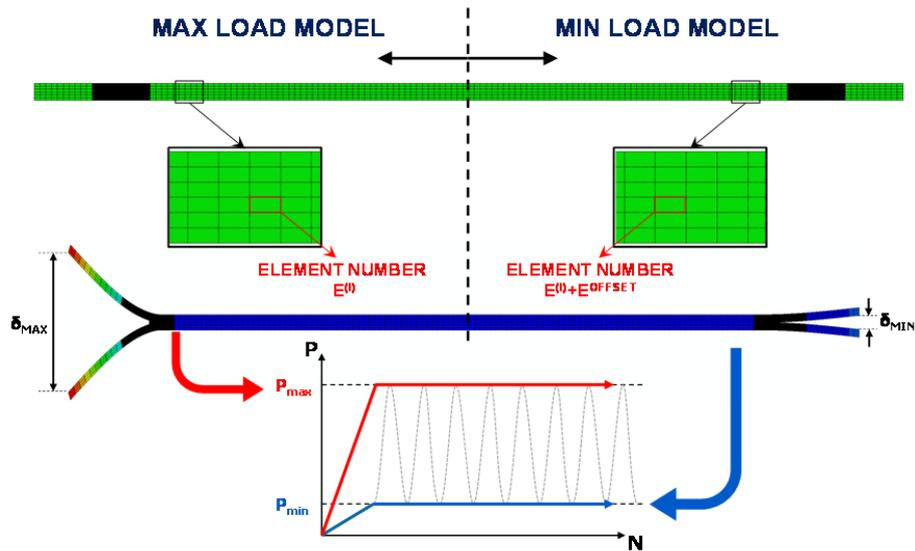
**Fig. 3 FE application of Min-Max Load Approach.**
