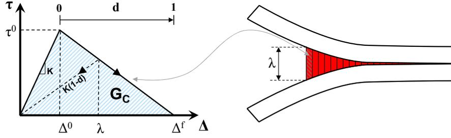
**Fig. 1 Constitutive response for traction-separation cohesive elements.**
