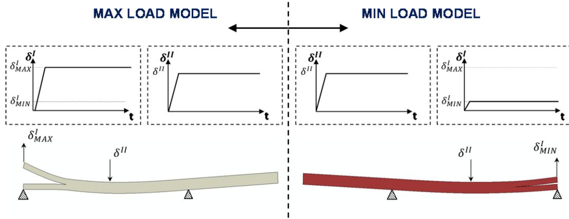
**Fig. 12 Min-Max Load Approach for modified MMB specimen.**
