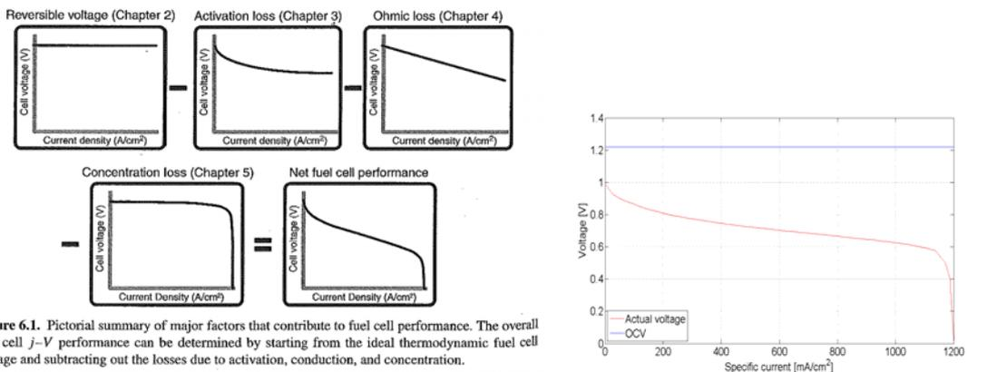
Figure 9 Build-up of FC characteristic, ref [16] (left) and FC characteristic from model (right).
