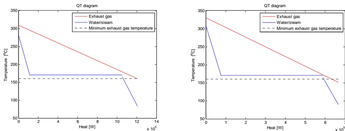
Figure 6 Q-T diagram for design condition (left) and reduced load (right). The
