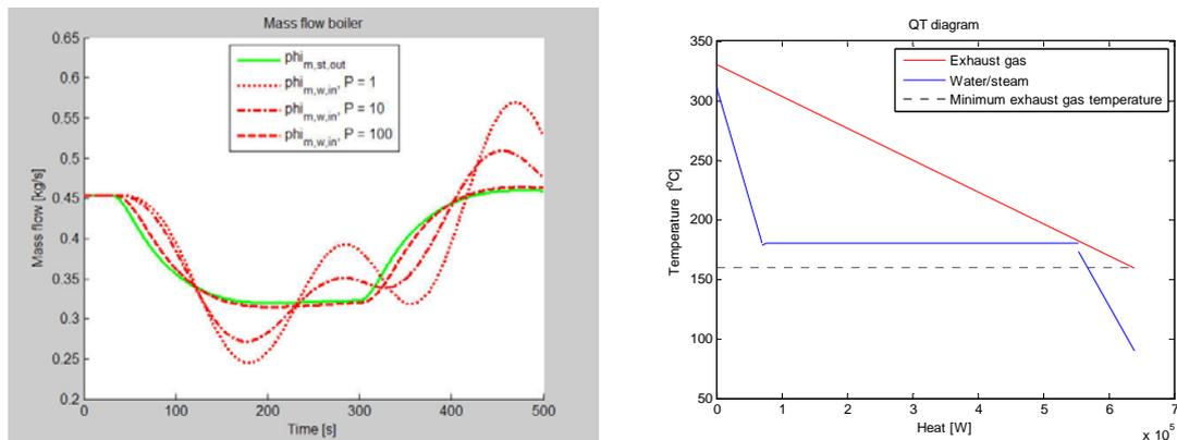
Figure 8 Feed water mass for different proportional gain settings (left) and Q-T diagram for reduced load and increased pressure (right)
