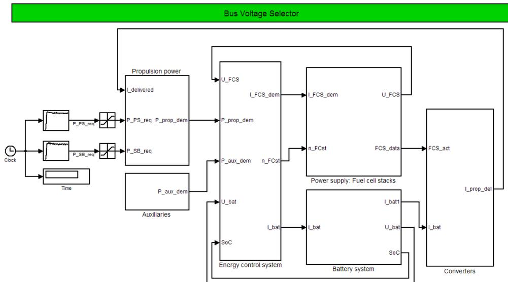
Figure 10 Top layer of hybrid FC system
