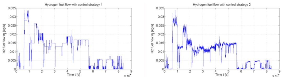
Figure 11 Hydrogen fuel flow with more energy efficient control strategy on the right
