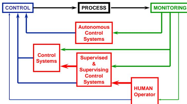
Figure 2 Control & Monitoring: layers and levels
