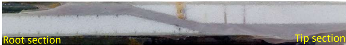
Figure 5.4: Picture of cut web joint, designed bondline thickness was 6 mm and achieved bondline thickness was 5-8 mm.
