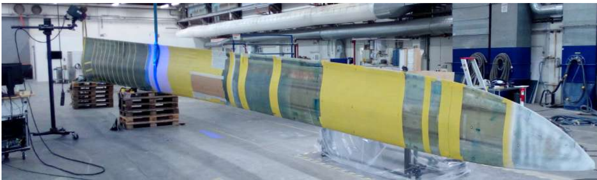
Figure 3.10: Picture of TA being scanned with LE down. Pallets only support the former root section, cranes to keep TE up. Tape was applied on the surface for the scanner to work properly
