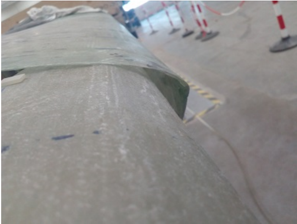
Figure B.4: Picture of not-fitting LE glue flange, this prevented adjusting the tip to the correct position
