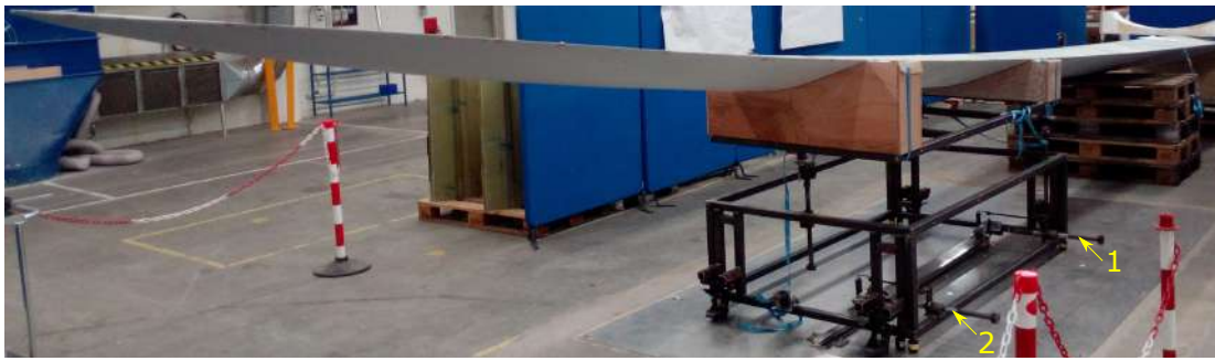
Figure 2.2: Picture of aligned LM42.1 tip, cut position is in between six-axis manipulator and stack of pallets.
