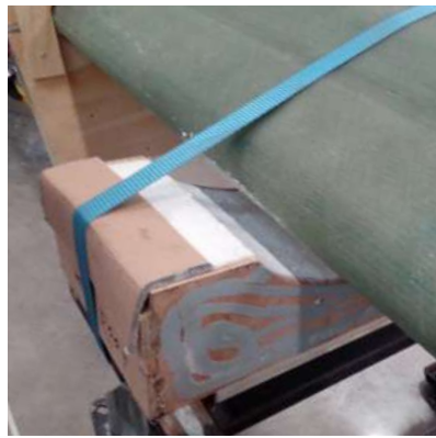
Figure 3.9: Picture of TA tip being pushed out of the supported position.
