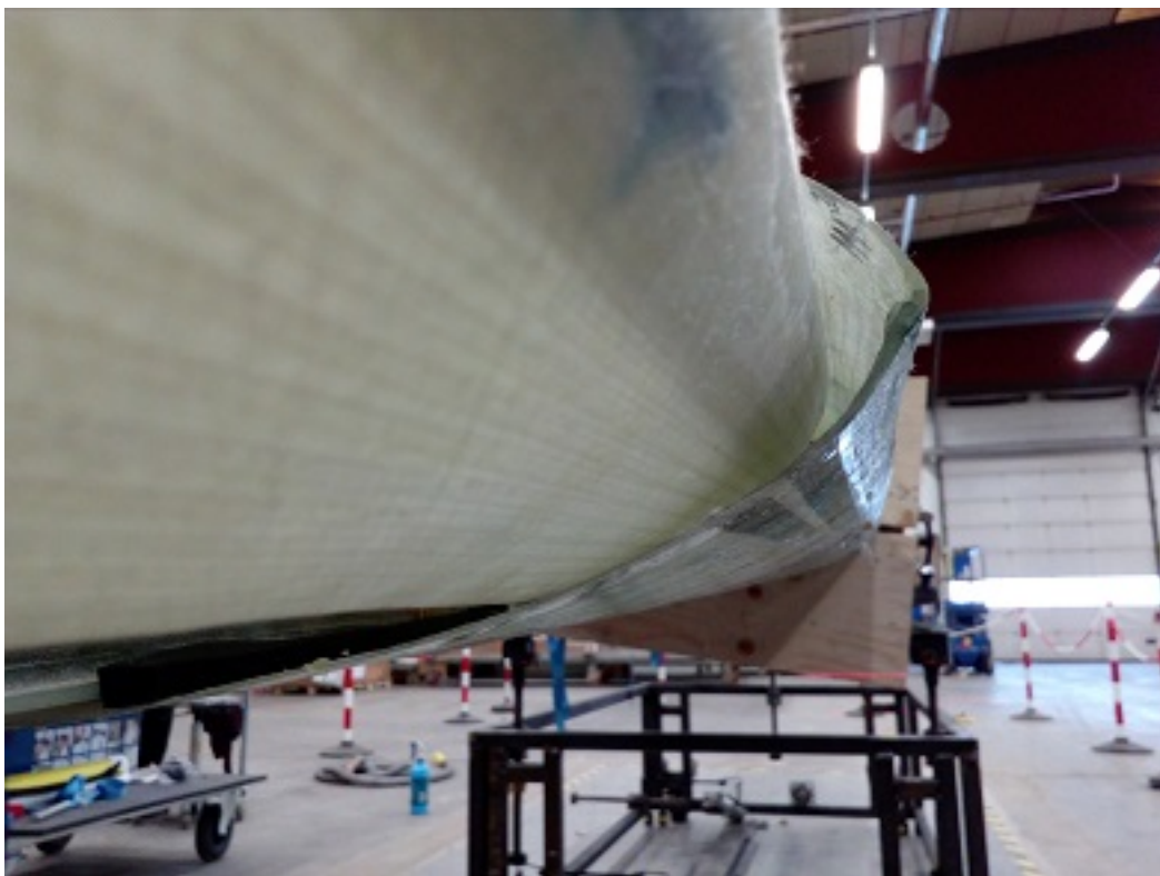
Figure B.5: Picture of not-fitting LE glue flange, the cavity in-between the shell and flange was 32 mm, whereas the design was a constant cavity of 3 mm.
