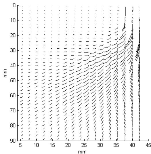
Figure 6: Displacement trajectories in 1g test.
