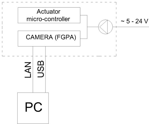
Figure 7: In-flight centrifuge camera-PC connection. LAN and USB ports are used to connect the PC and the camera. In-flight circuit providing 5 – 24 V is shown.
