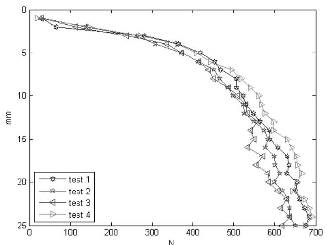
Figure 2b: Model footing installation. Ratio  $D/d_{50} = 28$ .
