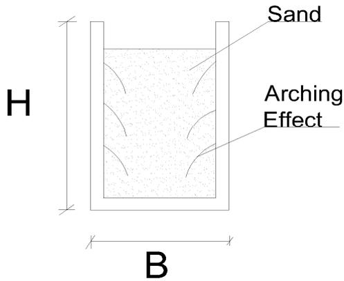
Figure 1: The silo effect with soil arches.
