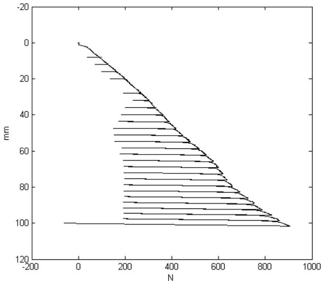
Figure 3: Pile head load during jacked installation
