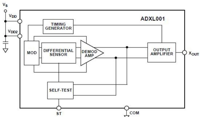
Figure 8: Functional diagram for Analog Devices ADXL001 MEMS accelerometer.
