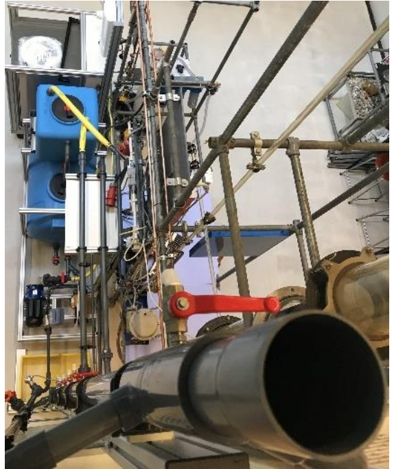
Figure 12 Column top view D = 57 \text{ mm} , L = 4 \text{ m}
