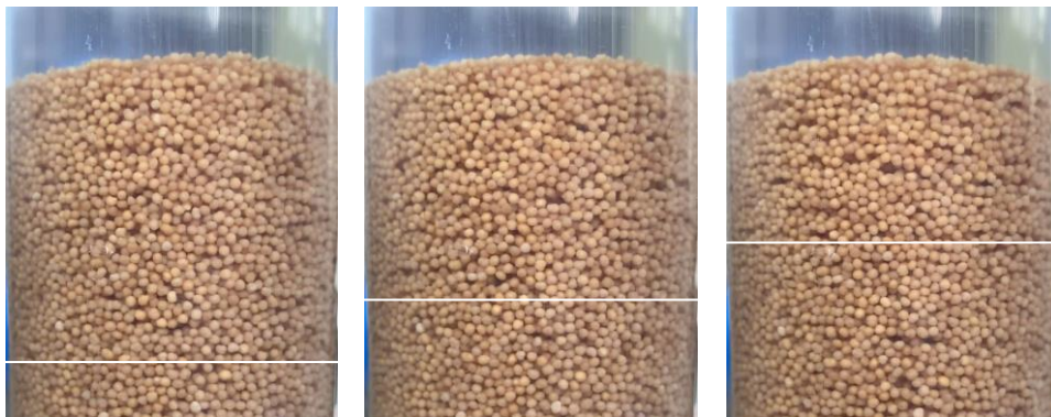
Figure 66 Sequence of 1.4-1.7 mm calcite pellets in a 57 mm column. Dark zones are caused by local pockets of water, v_s = 25 mm/s, \langle \epsilon \rangle = 0.50 m 3 /m 3 , average interstitial fluid velocity 50 mm/s. White lines represent the progression of waves of voids moving up at 50 mm/s. The time interval between images is 0.17 s, corresponding to 8.5 mm or 5.5 particle diameters. The wave progression can be seen more clearly on the provided video material (Kramer et al., 2020e; Kramer et al., 2020h).
