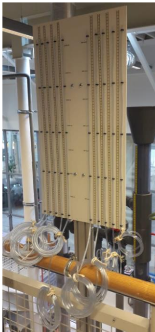
Figure 17 Hydrostatic measurement board with longitudinal taps
