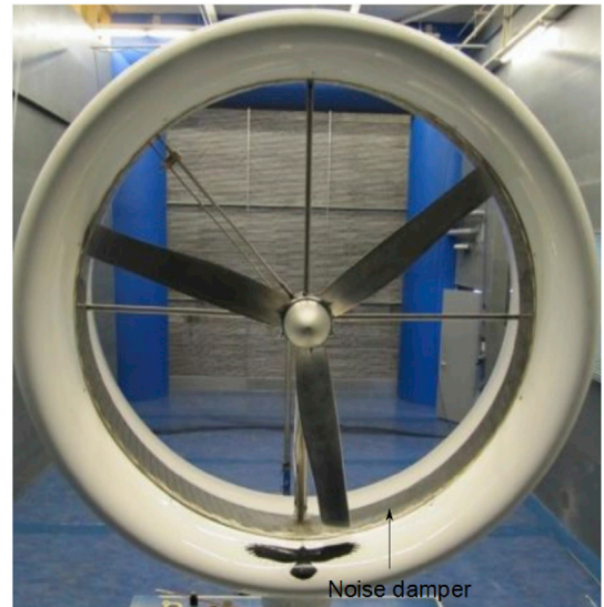
Fig. 7. Front view of the DonQi® DWT model used for the experimental study (Ten Hoopen, 2017).
