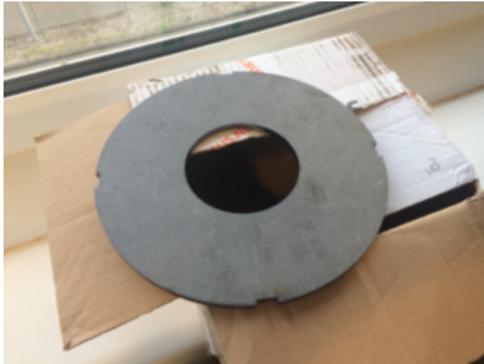
Fig. 7.10 Hot-rolled SA2.5 steel ring shear sample
