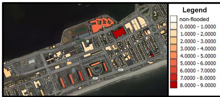
Figure 4-12 - Impression of the spatial distribution of the inundation depth indicator
