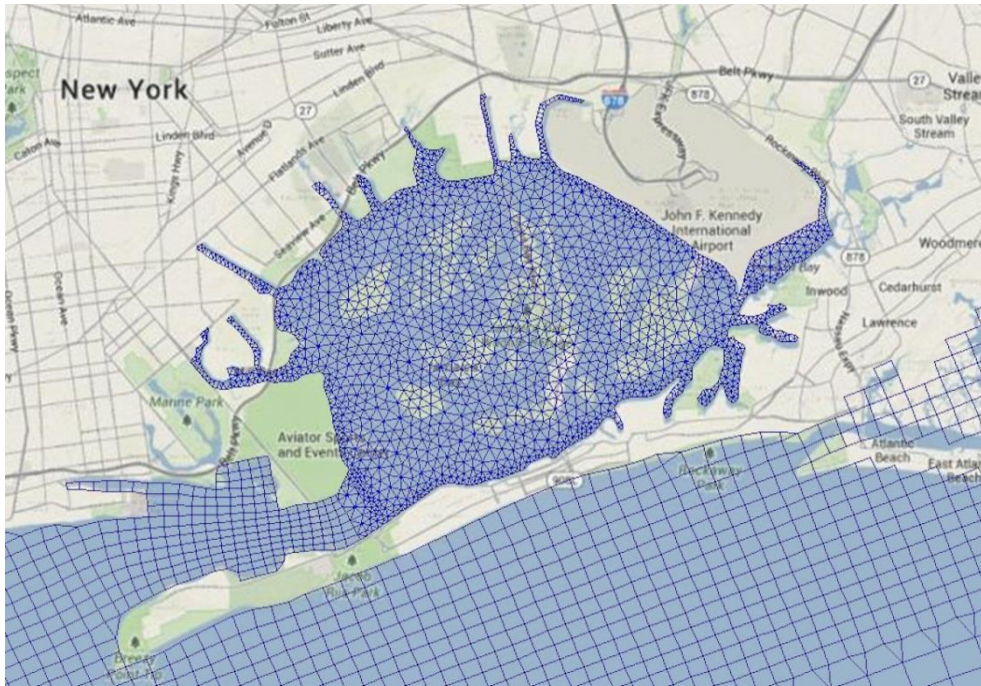
Figure 3-23 - Grid configuration in the Jamaica Bay and around the Rockaway Peninsula.
