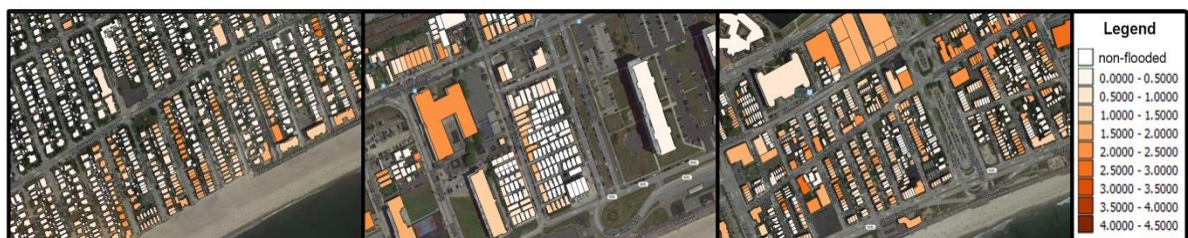
Figure 4-18 - three Impressions of the spatial distribution of the flow velocity indicator
