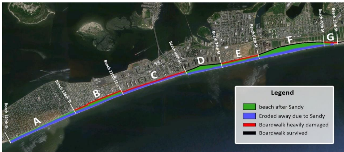
Figure 2-14 - Overview of damage to the beaches and Boardwalk; based on aerial pictures taken directly after the storm.
