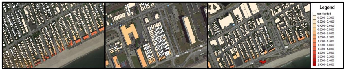
Figure 4-16 - three Impressions of the spatial distribution of the wave attack indicator
