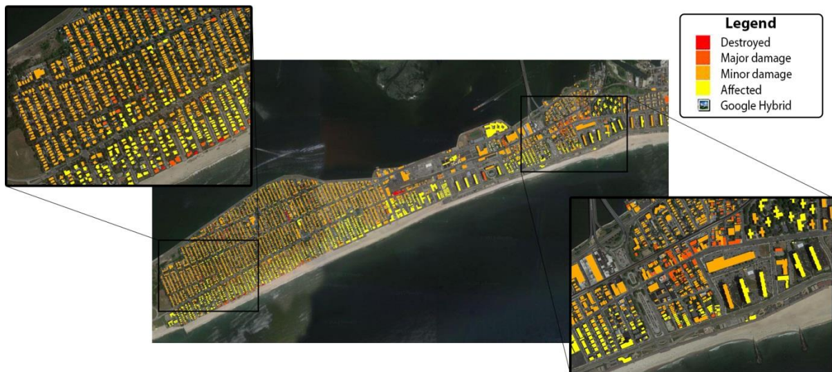
Figure 2-21 - Spatial representation of the ImageCat damage Analysis
