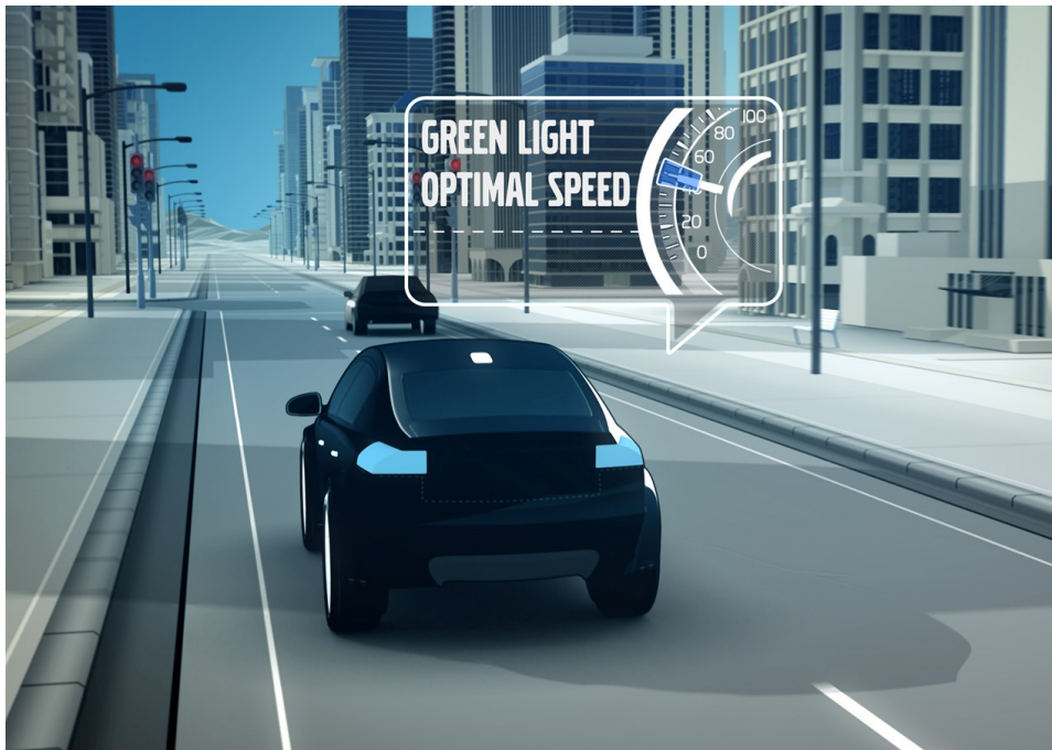
Figure 1.2: Visualization of green light optimal speed advice (GLOSA) [49]. The vehicle is approaching a red signal at an intersection and receives a speed advice that ensures it arrives when the signal has turned green.
