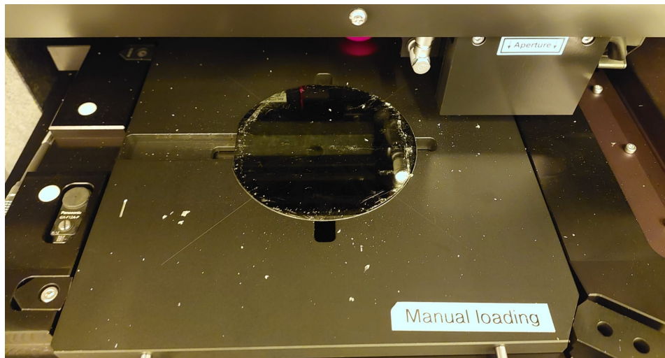
Figure 5.11: The result of pneumatic focusing on the PDMS substrate on PFOTCS. PDMS particles are spread everywhere due to the pneumatic airflow.
