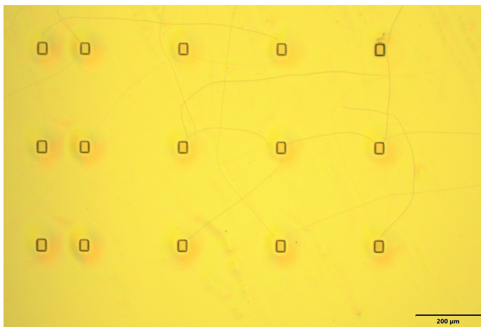
Figure F.1: Cracking behavior of PDMS after high power (>70W) O 2 plasma treatment.
