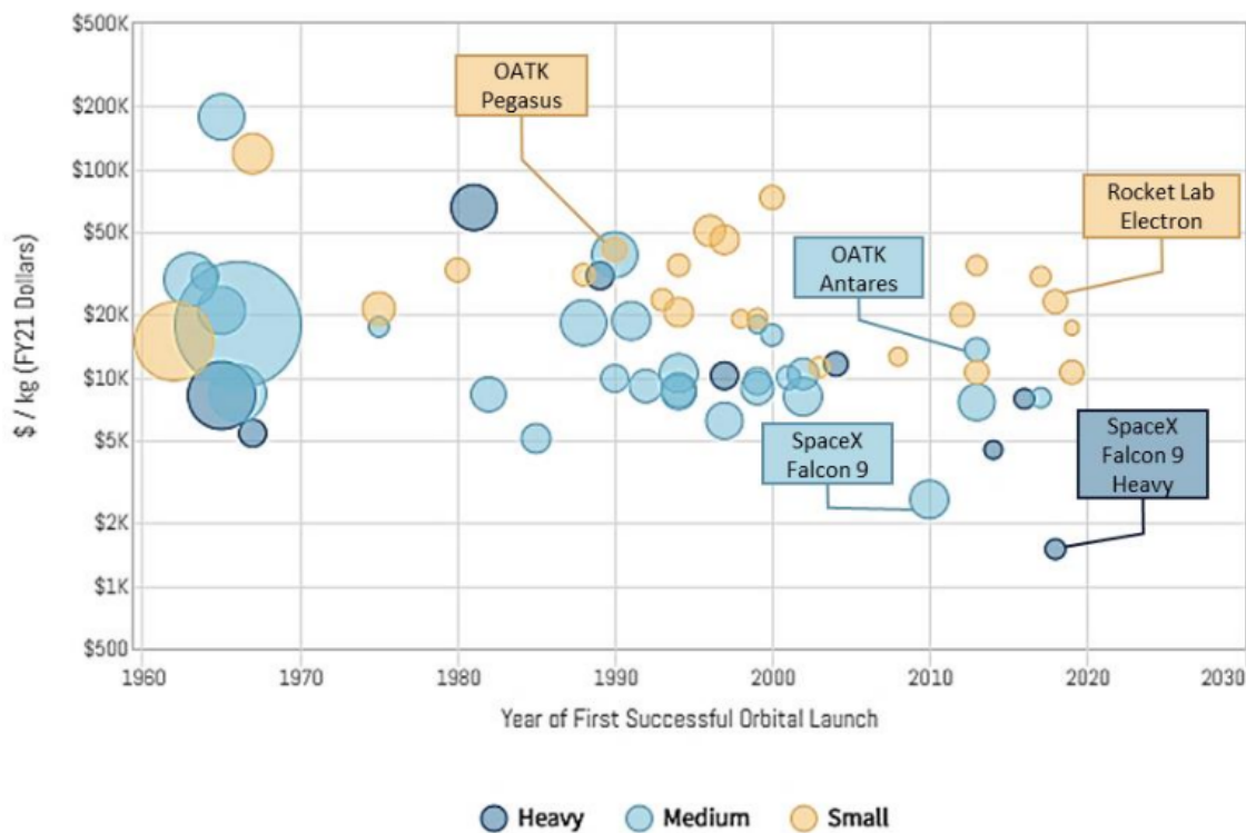
Figure 1.5: Launch cost per kilogram versus year of launch in different vehicles (Roberts & Kaplan, 2022).
