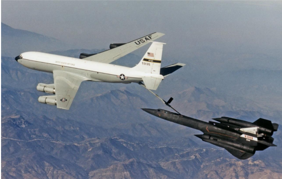
Figure 1.1: Aerial refueling of an SR-71 Blackbird aircraft by a tanker plane (M. A. Luu & Hastings, 2022).
