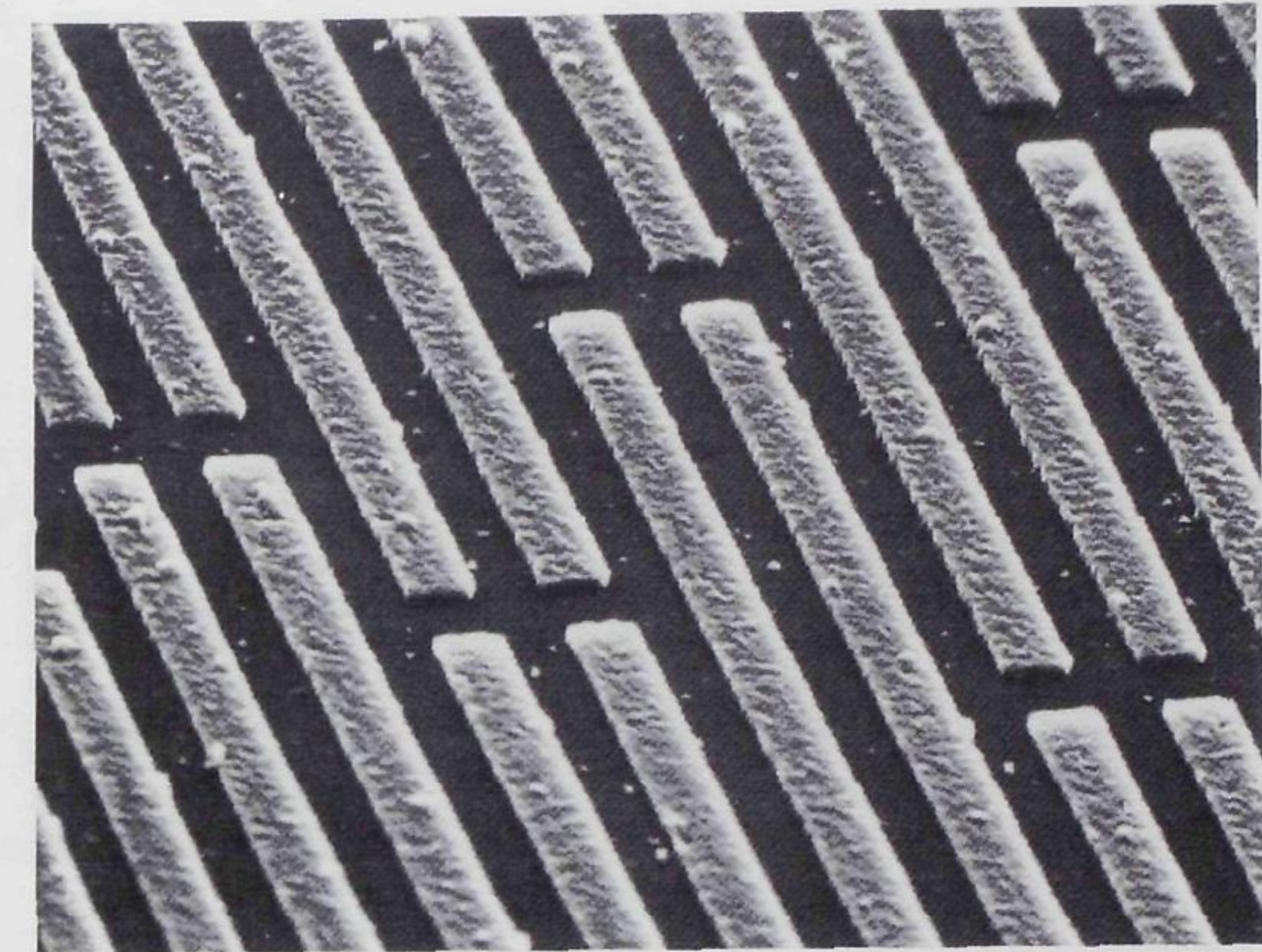
Figure 4.5: Aluminum electrode structure (1 \mu\text{m} electrode width).
