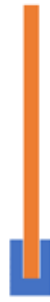
Figure H.22: A schematic example of the influence of the tip design with respect to the screw for the maximum amount of FLE to take place. Here the fit is perfect thus no FLE is mechanically possible to take place. However, a perfect fit limits the ability to rotate the tip with respect to the fiducial screw.
