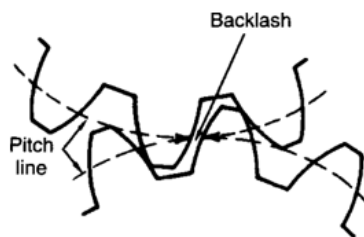
Figure H.14: A schematic example of the mechanical backlash gap between mating teeth of two gears (2022).
