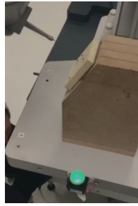
Figure 5.13: An example of the LED placement and visual feedback to the operator. Here the colour is green, meaning the robot is in fixed or safety mode.
