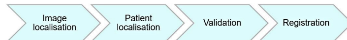
Figure 1.4: A schematic outline of the steps to execute patient-to-image registration. First, locate the landmarks or PC in the image space. Then locating the identical landmarks or another PC in the patient or robot space. Validation of the localisation methods is required, whereafter registration can be executed, resulting in a transformation matrix.
