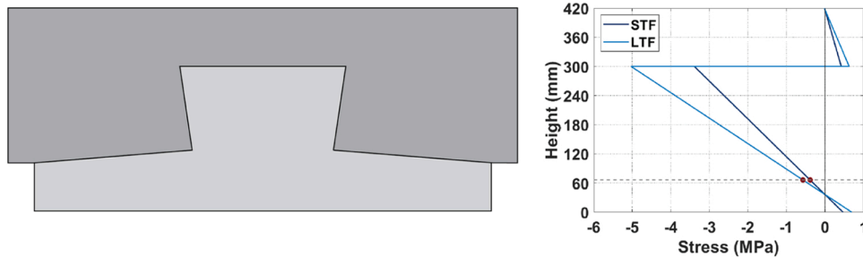
Fig. 17. Stress distribution in the middle of cross-section due to restrained shrinkage on STF and LTF.
