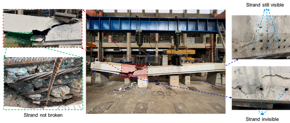
(b) LTF: Anchorage failure
