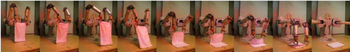
**Figure 2-3:** The successful motion of a dual-arm robot folding a towel with markers. [5]
