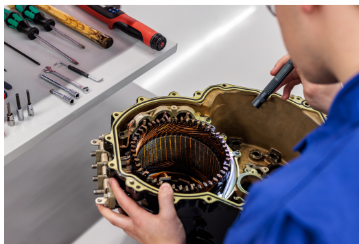
Figure 1.1: Technician working on an IDG unit in the Power Generation shop of the component maintenance provider.
