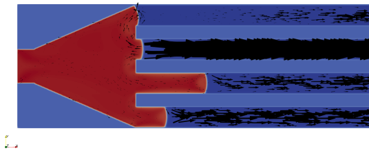
Figure 6.20: Multi channel simulation showcasing numerical explosive boiling simulation with R = 1 , \sigma = 0.30 and a = \frac{3}{49} at \Delta t = 1020e3
