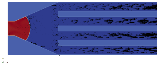
Figure 6.15: Multi channel simulation showcasing numerical explosive boiling simulation with R = 1 , \sigma = 0.30 and a = \frac{3}{49} at \Delta t = 120e3
