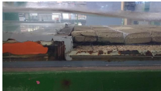
Figure 3.2: Detail of the transition between the stilling basin and the block mattress
