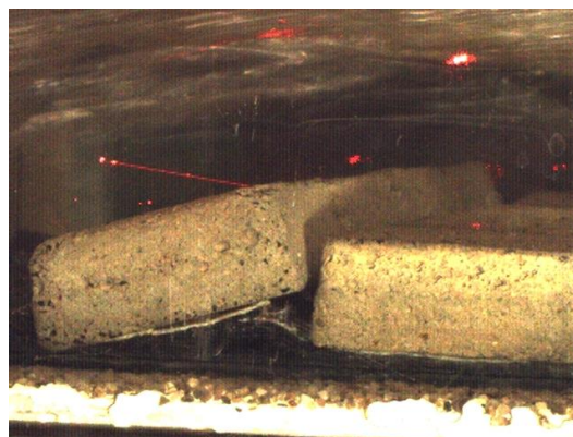
Figure 4.3: Failure of the last row of the block mattress
