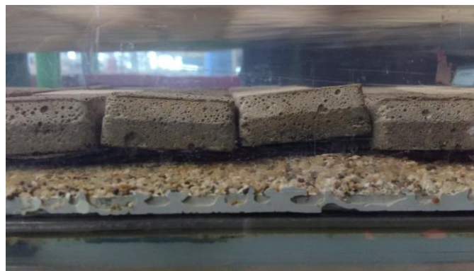
Figure 4.12: Displacement of the middle block limited by the cohesion supplied by the adjacent blocks. Unlike the edge situation, in the middle of the mattress, the blocks are surrounded by blocks downstream and upstream.
