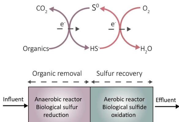
Fig. 3. Schematic diagram and flow chart of internal sulfur cycling (ISC) process.
