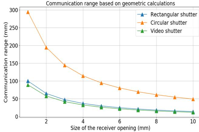
Figure 6.7: Computed value of communication range based on size of receiver opening.
