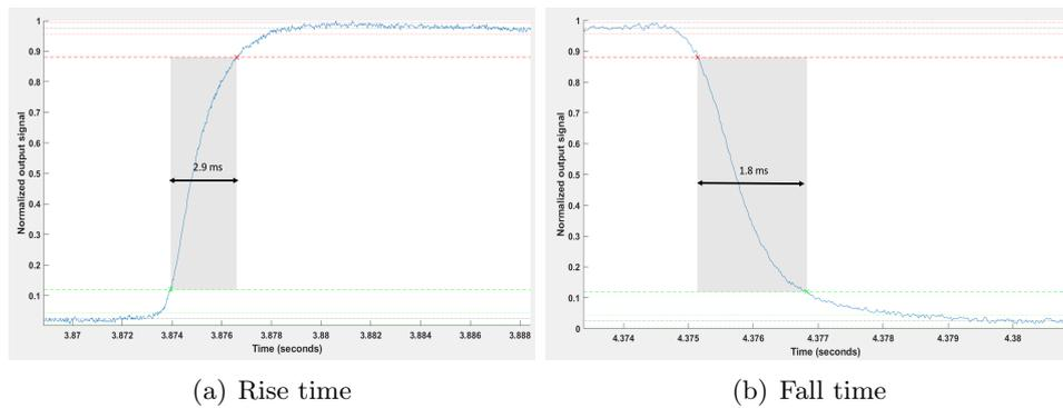
Figure 4.5: Rise and fall times of the video shutter at 5V.
