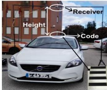
Figure 2.3: Setup of a barcode based passive communication channel [23] .
