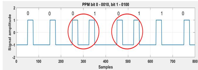
Figure 6.12: PPM for ASCII synchronization character 22.
