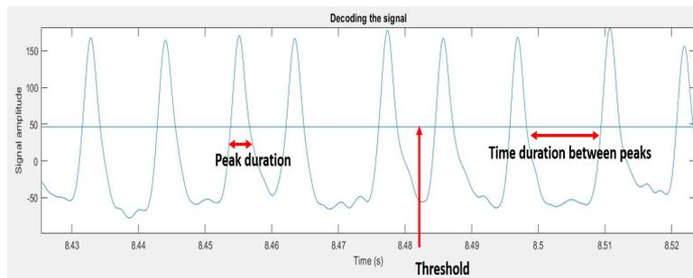
Figure 6.1: Signal measurements for decoding.
