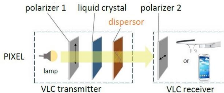
Figure 2.9: Indoor positioning system using color based light modulation [30].
