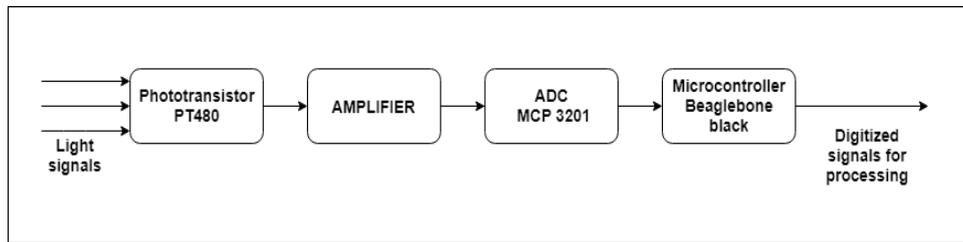
Figure 3.4: Block diagram depicting the structure of the receiver.
