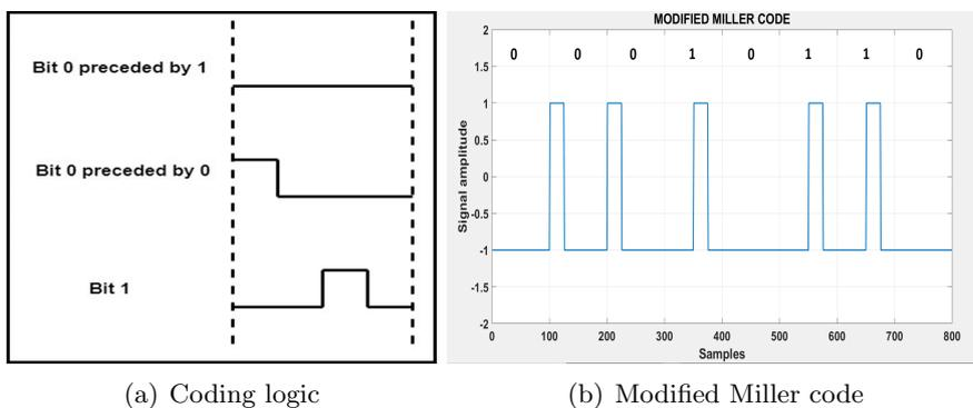
Figure 5.6: Modified Miller coding for bit sequence 00010110.
