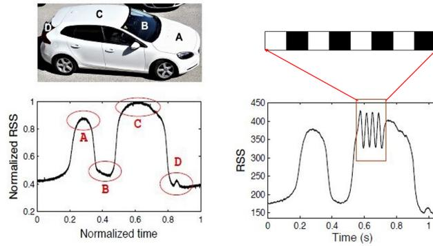
Figure 2.4: Shape of the car detected by the receiver (left) and the variations of the barcode captured when placed on the roof of the car (right) [23] .
