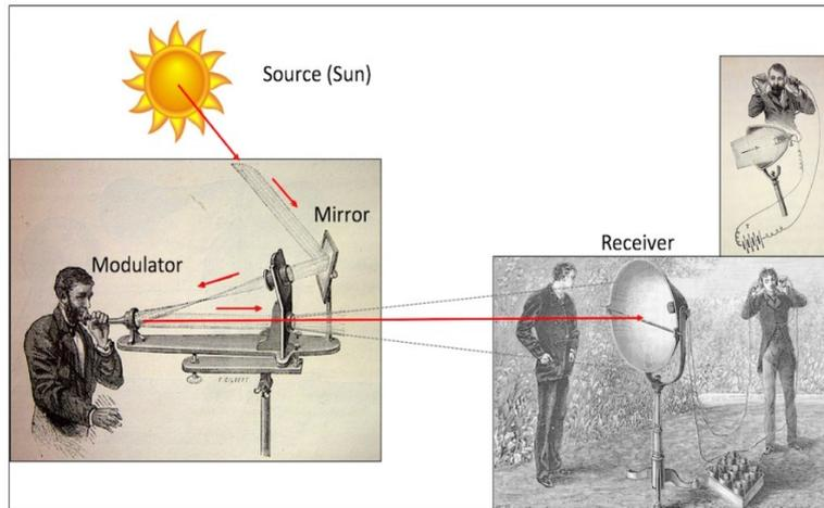
Figure 1.2: Illustration of the working of a photophone [7].
