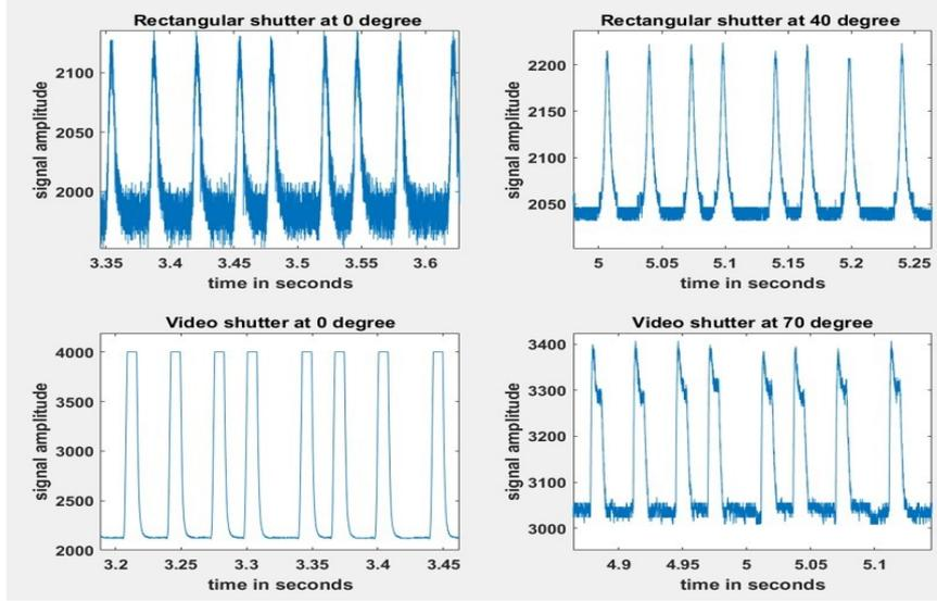
Figure 6.5: Received PPM signal for varying orientation angles of shutters.
