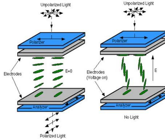
Figure 3.2: Output states of the liquid crystal (LC) shutter- translucent (left) and opaque (right) [15].
