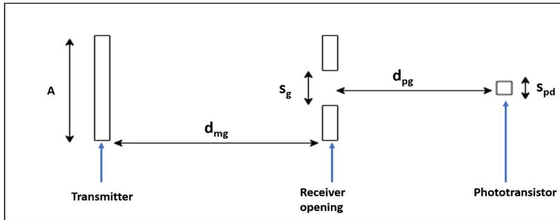
Figure 6.6: Parameters used for theoretical range calculation.
