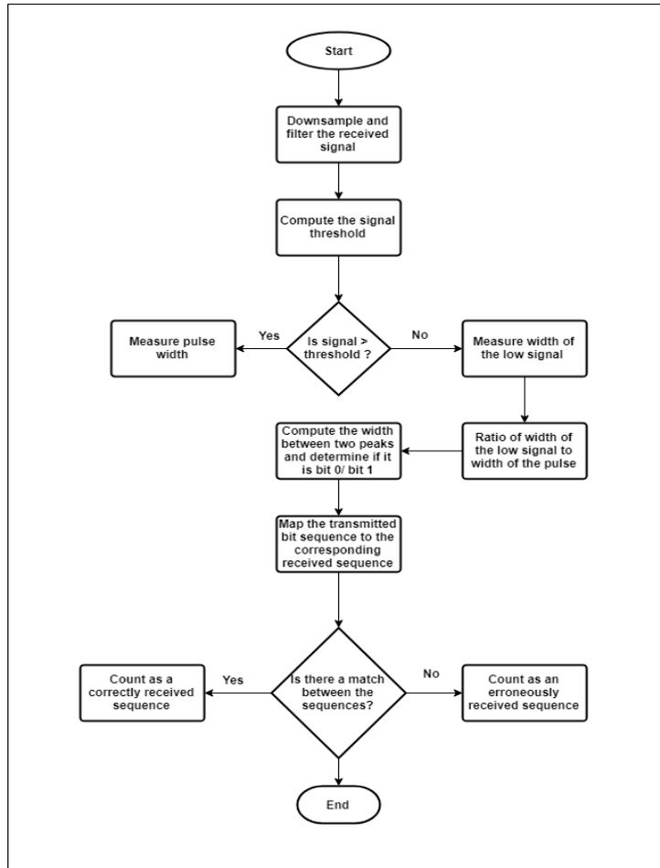
Figure 6.2: Flowchart representing the approach to demodulate the PPM received signals from the LC shutters.
