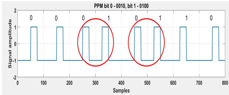
Figure 5.12: PPM type 2 - the minimum width between pulses is 50% of the bit period (shown by the red circle).
