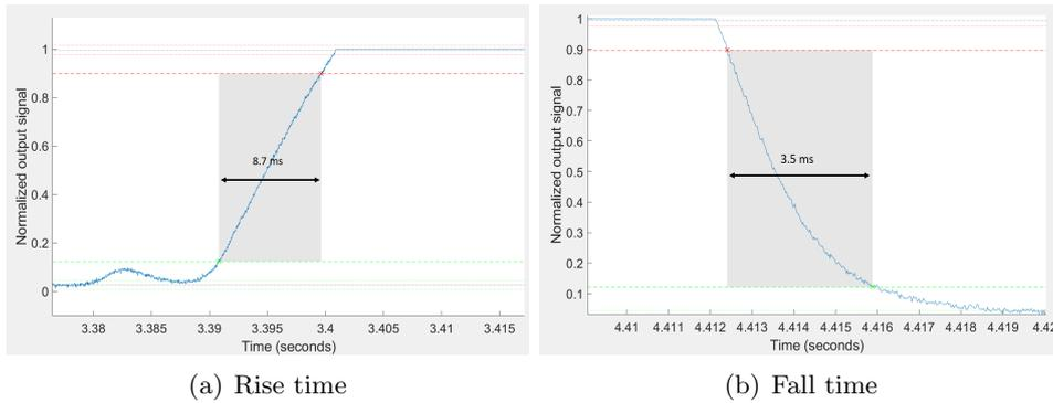
Figure 4.3: Rise and fall times of the rectangular shutter at 5V.
