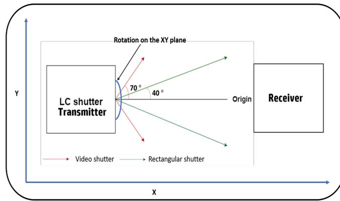
Figure 6.4: Orientation angle of the LC shutter with respect to the receiver.
