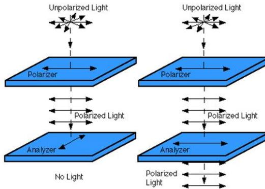
Figure 2.7: Output of the polarizer- no light exiting analyzer (left) and polarized light exiting analyzer (right) [15].
