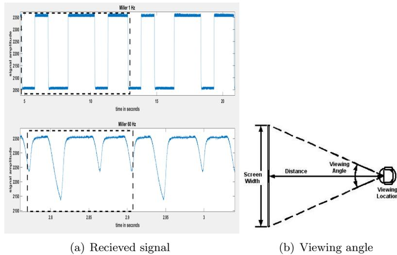
Figure 5.5: OOK with Miller coding for rectangular shutter with the polarizer placed at the receiver.
