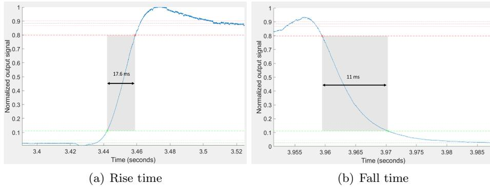
Figure 4.4: Rise and fall times of the circular shutter at 5V.
