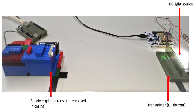
Figure 4.1: Experimental setup with the transmitter (right) and the receiver (left).
