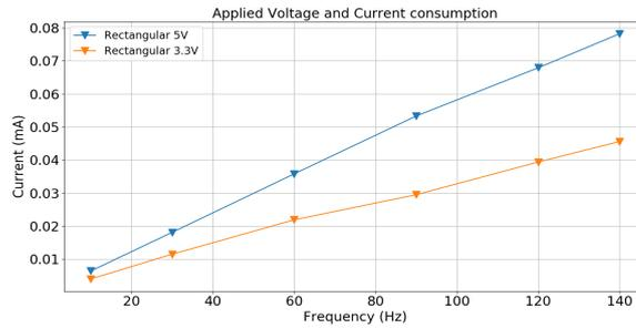
Figure 6.10: Relation between current consumption and supply voltage-Rectangular shutter.
