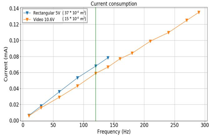
Figure 6.9: Relation between the frequency and current consumption for the shutters.
