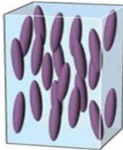
Figure 3.1: Nematic liquid crystal molecules - parallel along the longer axis [3].
