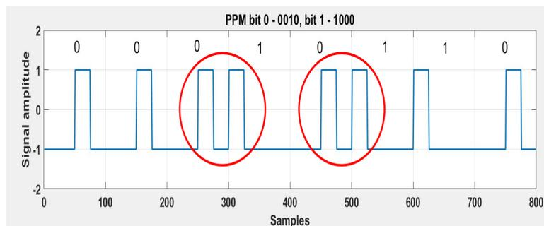
Figure 5.11: PPM type 1 - the minimum width between pulses is 25% of the bit period (shown by the red circle).
