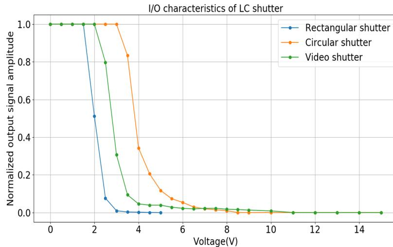
Figure 4.2: Normalized output signal amplitudes for different LC shutters.
