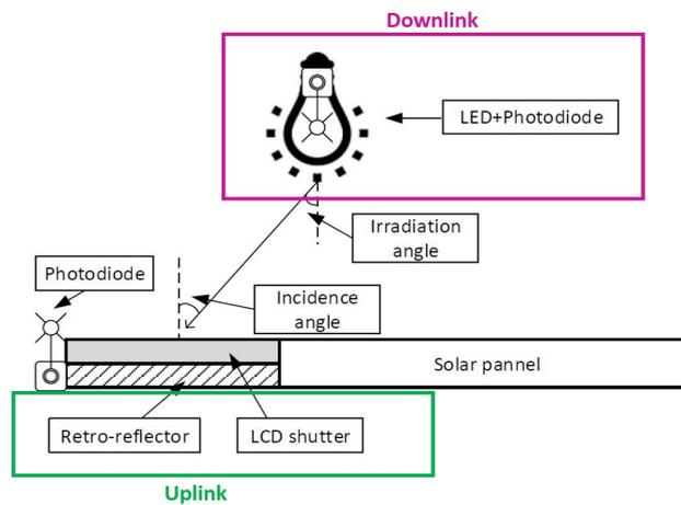
Figure 2.8: Bidirectional visible light communication with backscattered light [14].
