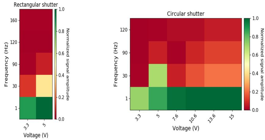
(a) Amplitude variation of rectangular shutter (b) Amplitude variation of circular shutter
