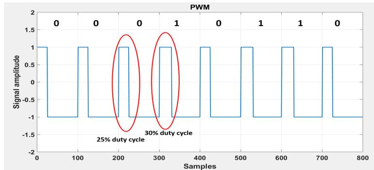
Figure 5.8: Pulse Width Modulation (PWM).
