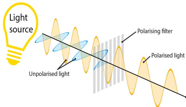
Figure 2.6: Polarization of light [5].
