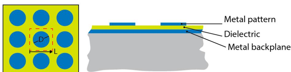
**Figure 2.** Schematic of a metamaterial structure.
