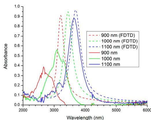
**Figure 4.** Expected and measured the absorbance of mid-infrared metamaterial absorbers. Finite difference time domain (FDTD) analysis was used to simulate the response of the ideal metamaterials to the incident electromagnetic wave.
