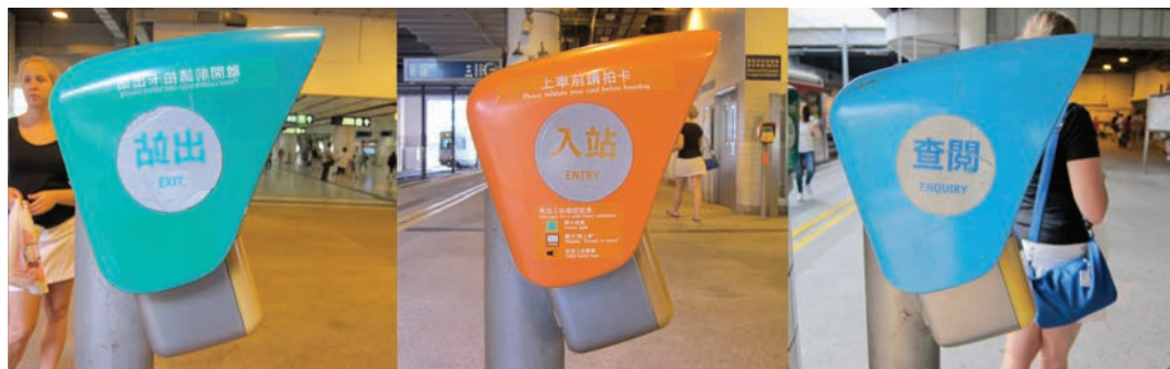
Figure 27: Side-view of lightrail validators in Hong Kong. From left to right: Exit, Entry, and Enquiry.
