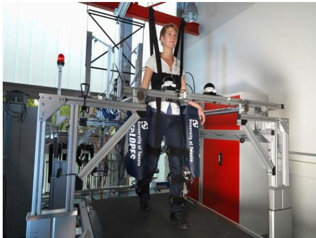
Figure 15: The Lopes is a bilateral exoskeleton with eight degrees of freedom. The actuators are detached from the exoskeleton and connected to the joints via Bowden cables and springs. The robot is impedance controlled via series elastic actuation.
