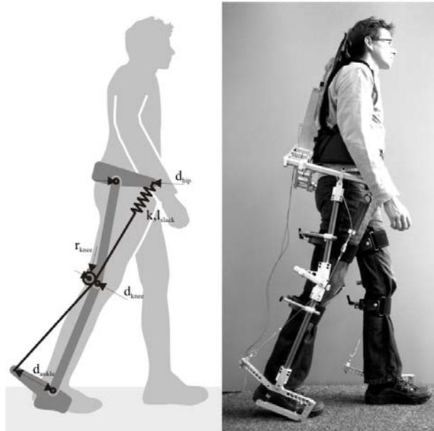
Figure 23: Left: Schematic drawing of the exoskeleton concept with artificial tendons (black). Right: A photo of the exoskeleton
