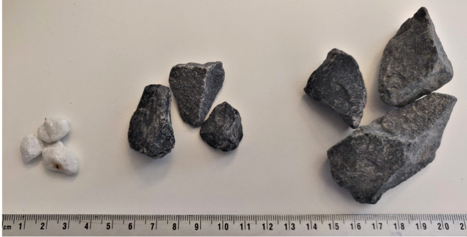
Figure 5.9: A sample of the three gradations used in Fontijn's lab tests. [30]
