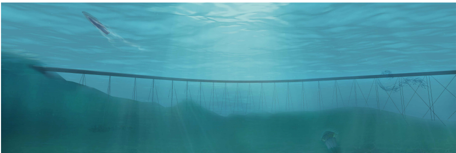
Figure 1.1: Sketch of submerged floating tunnel (CCCC SFT Technical Joint Research Team n.d.)
