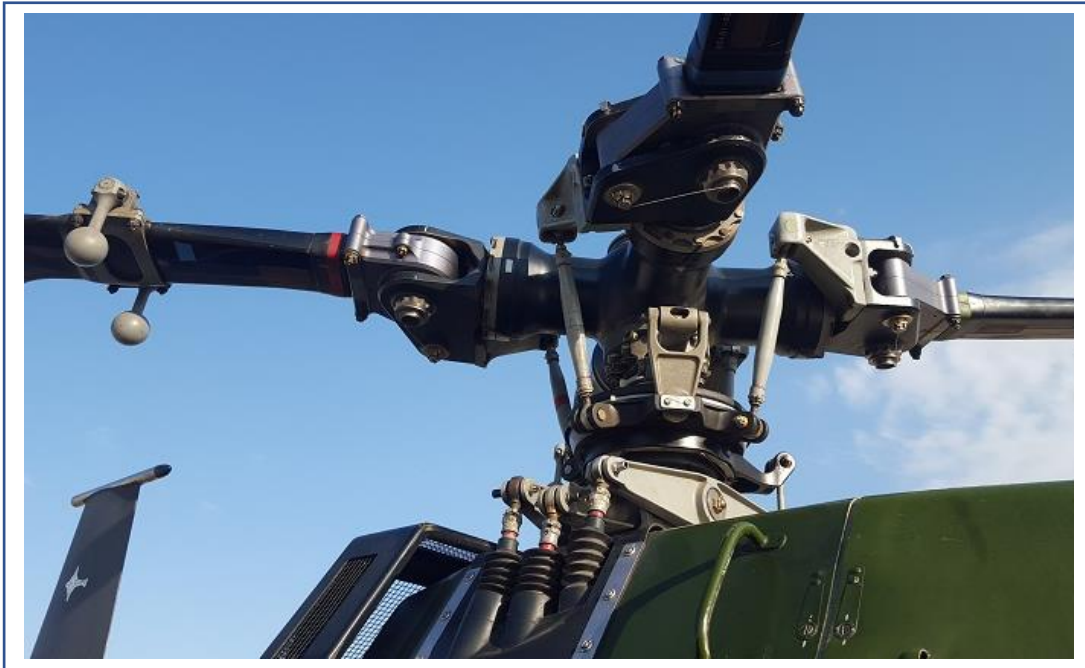
Figure C.5. The main-rotor assembly of the BO-105 helicopter. Each one of the blade is fitted with a pendulum absorber designed to alleviate vertical vibrations.
