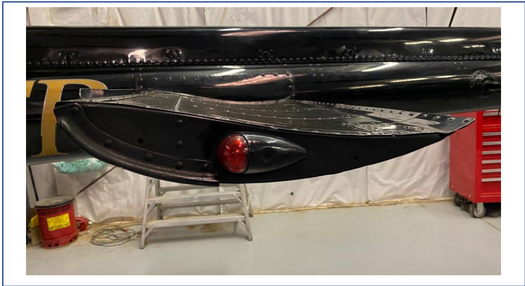
Figure C.3. The horizontal stabilizer. The horizontal stabilizer is designed to generate a down-loaded aerodynamic force in forward flight.
