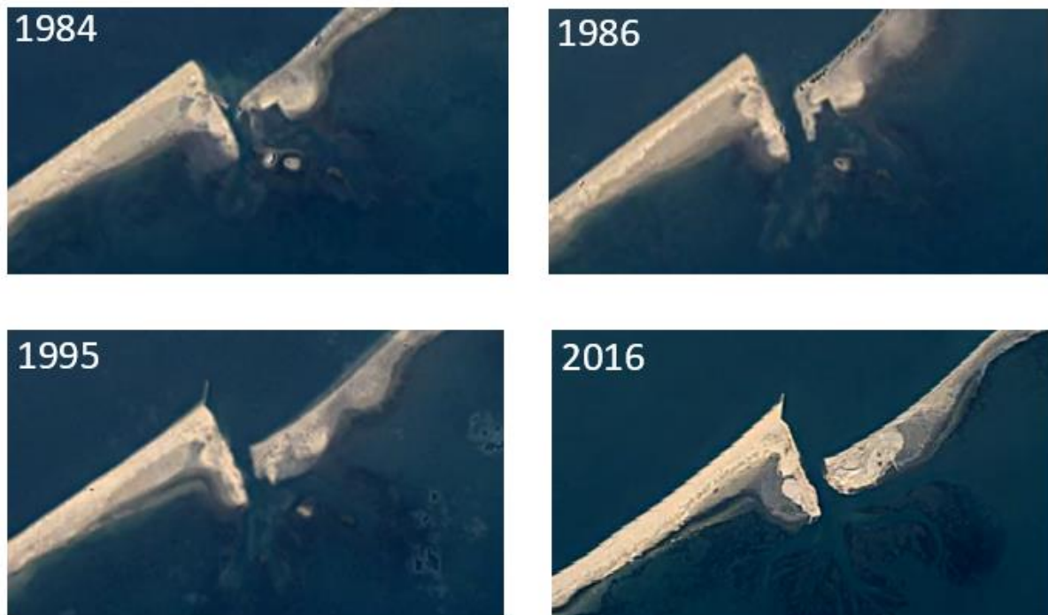
Figure 2-1: Evolution of Boughaz 1 inlet during 1984-2016. 1984: Instable system, 1986-1995: Breakwaters and maintenance dredging works, 2016: Current state("Lake Bardawil," 2015).
